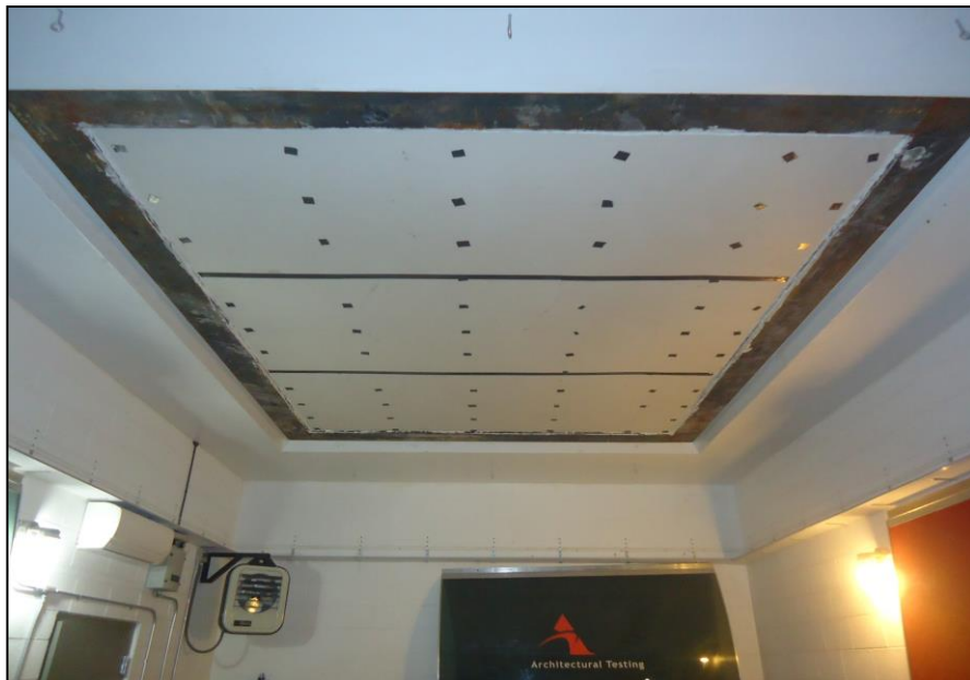
Receive Room View of Test Specimen Installation
