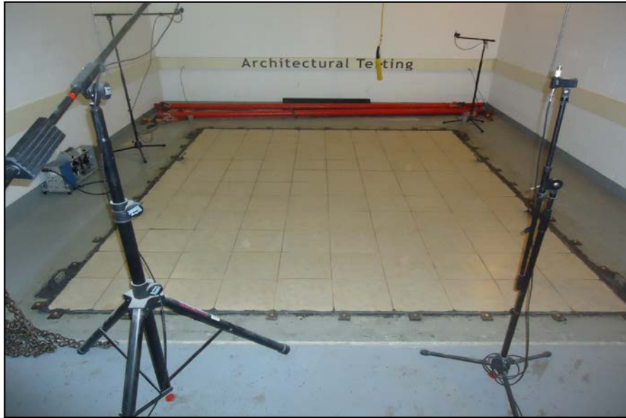
Source Room View of Test Specimen Installation
