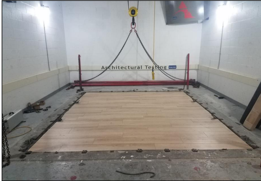
Source Room View of Test Specimen Installation
