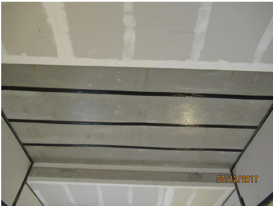
Figure 2 – Concrete slabs mounted in the test opening.
