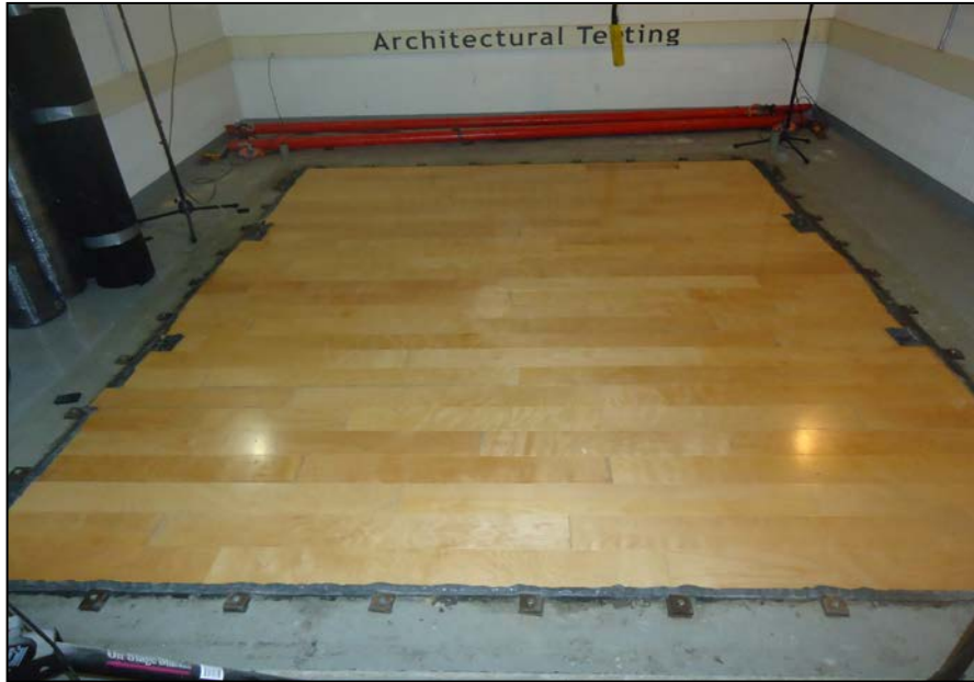
Source Room View of Test Specimen Installation
