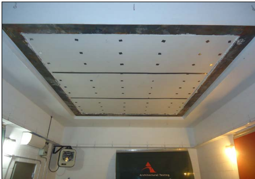
Receive Room View of Test Specimen Installation
