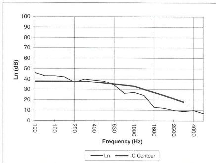
L<sub>n</sub> = Normalized Sound Pressure Level, dB
