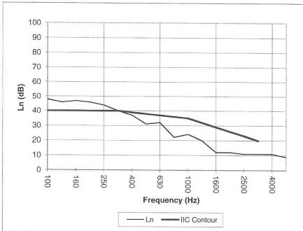
L<sub>n</sub> = Normalized Sound Pressure Level, dB
