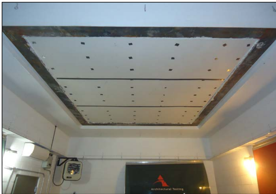
Receive Room View of Test Specimen Installation
