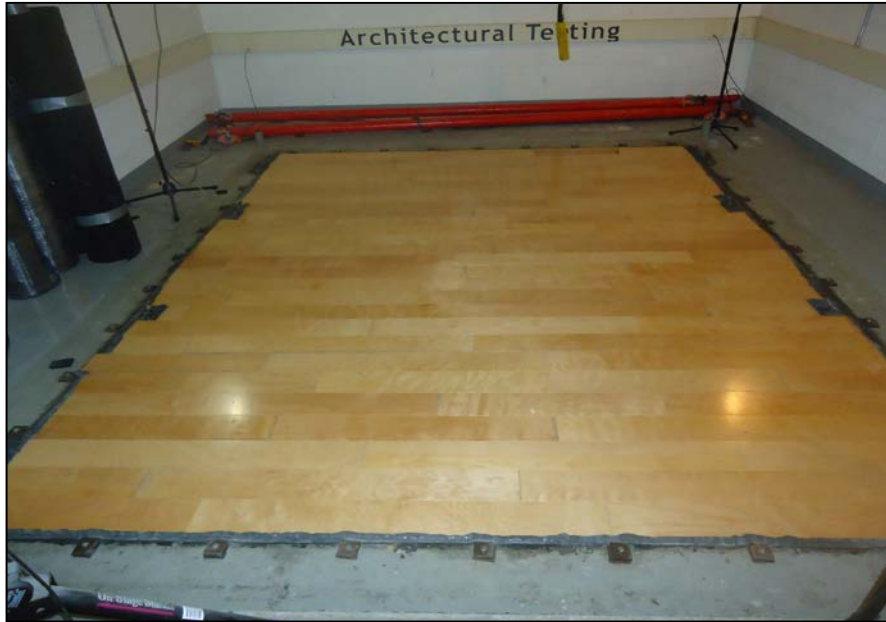
Source Room View of Test Specimen Installation
