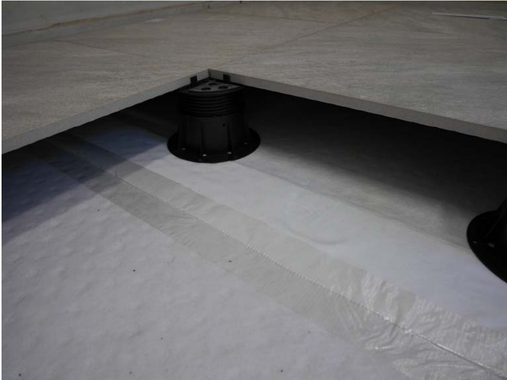
Figure B.4. Test setup during mounting: ceramic tiles on pedestals and Regupol® sound and drain 22.
