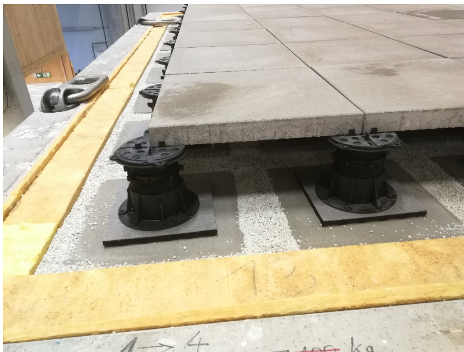
Fig. 3: The walk-on flat roof structure was decoupled from the test frame by means of impact noise insulation (TDPT 20, Saint-Gobain Rigips Austria GmbH).
