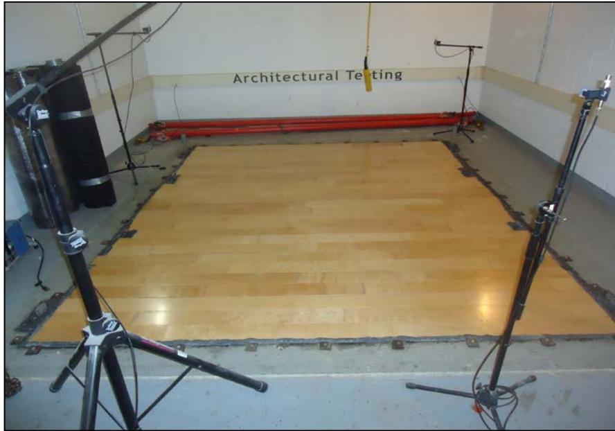
Source Room View of Test Specimen Installation
