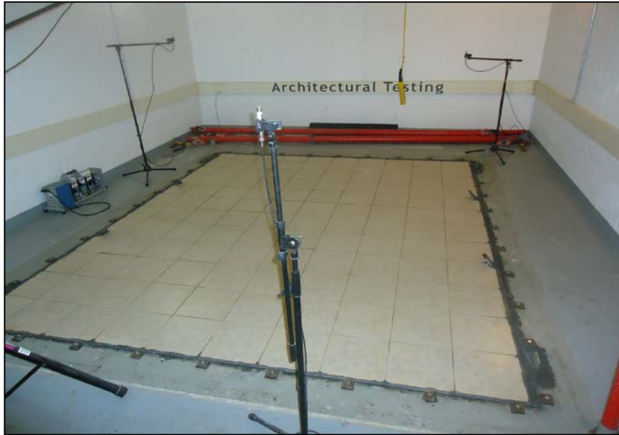
Source Room View of Test Specimen Installation
