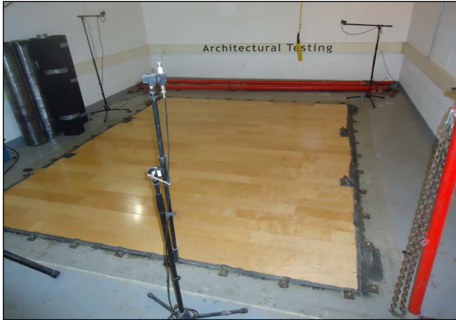
Source Room View of Test Specimen Installation
