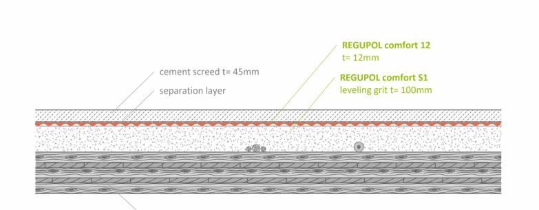
solid wood ceiling, 5 layers, t= 160mm, made of laminated wood ED-BSP, longitudinal layers t= 40mm, transverse layers t= 20mm
