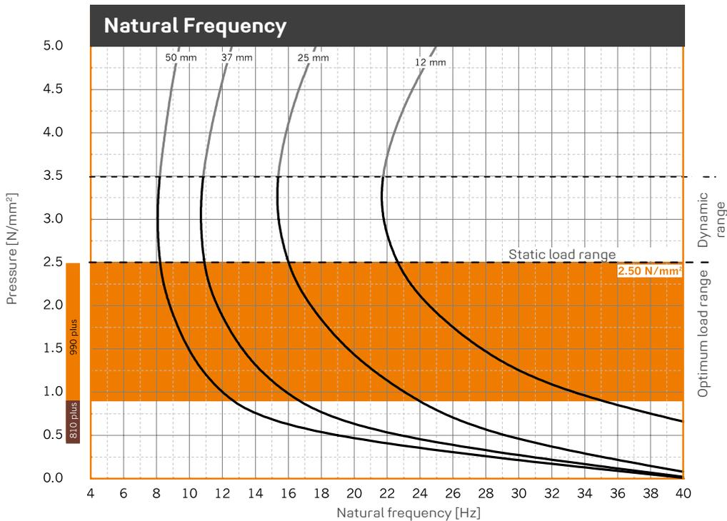
Natural frequency of a single-degree-of-freedom system (SDOF system) considering the dynamic stiffness of **REGUFOAM vibration 990plus** on a rigid base. Dimensions of test specimens 125 x 125 mm.
