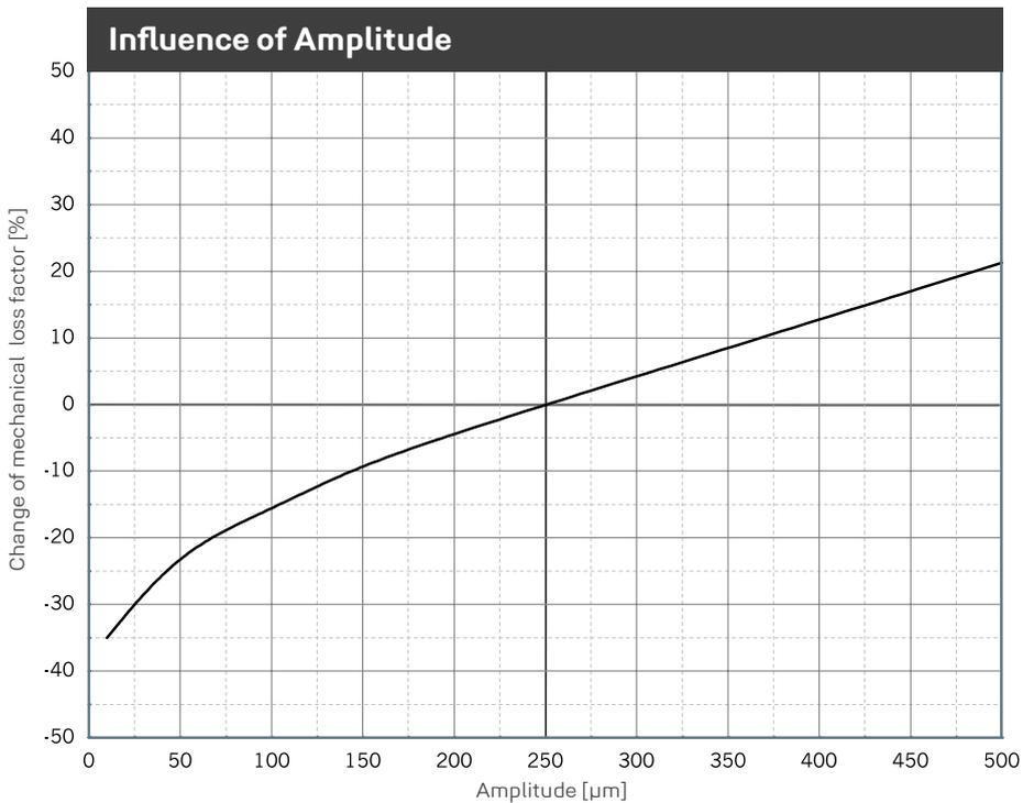
Change of the mechanical loss factor due to changes in amplitudes. Sinusoidal excitation at a constant mean load of 0.011 N/mm<sup>2</sup>, dimensions of the specimens 300 x 300 x 51 mm.
