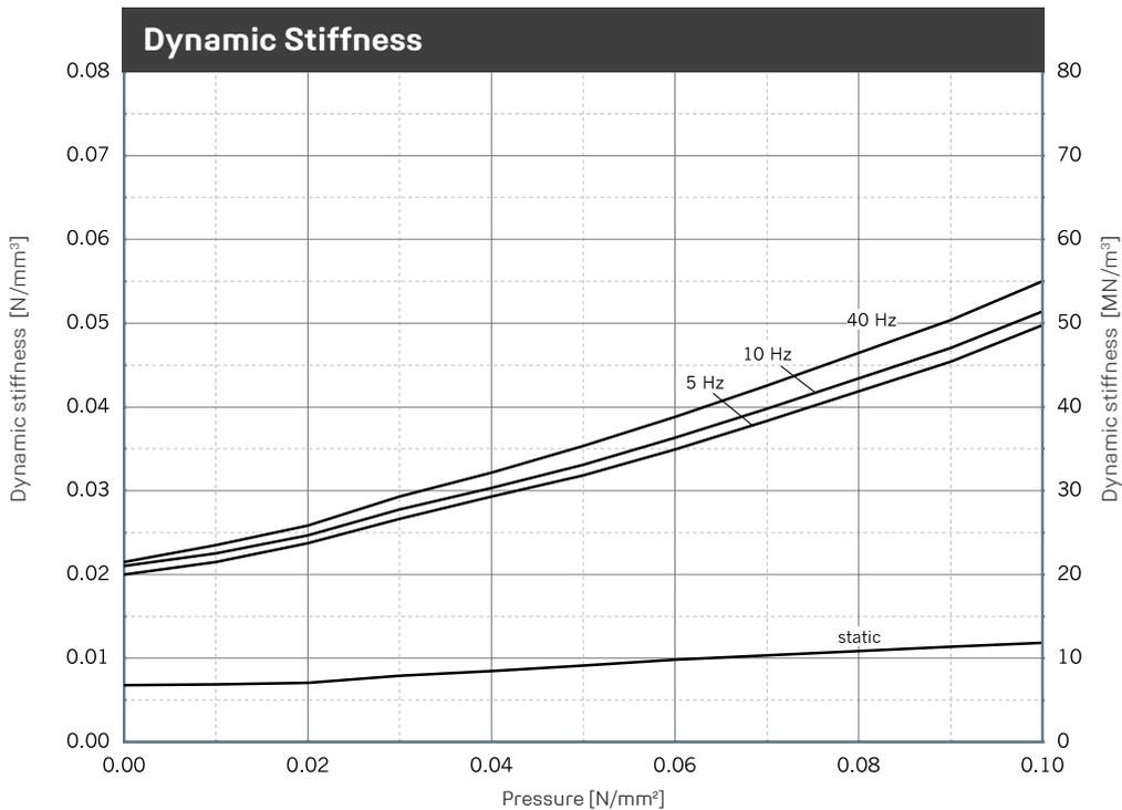
Illustration of the dynamic stiffness for sinusoidal excitation at a constant mean load and an amplitude of  $\pm 0.25$  mm. Dimensions of specimens 300 x 300 x 45 mm; static stiffness as a result of the tangent modulus of the spring characteristic. Tested in accordance with DIN 53513.
