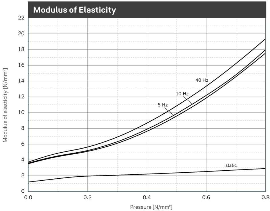
Illustration of the dynamic modulus of elasticity for sinusoidal excitation at a constant mean load and an amplitude of  $\pm 0.25$  mm. Dimensions of specimens  $250 \times 250 \times 40$  mm; static modulus of elasticity as a result of the tangent modulus of the spring characteristic. Tested in accordance with DIN 53513.
