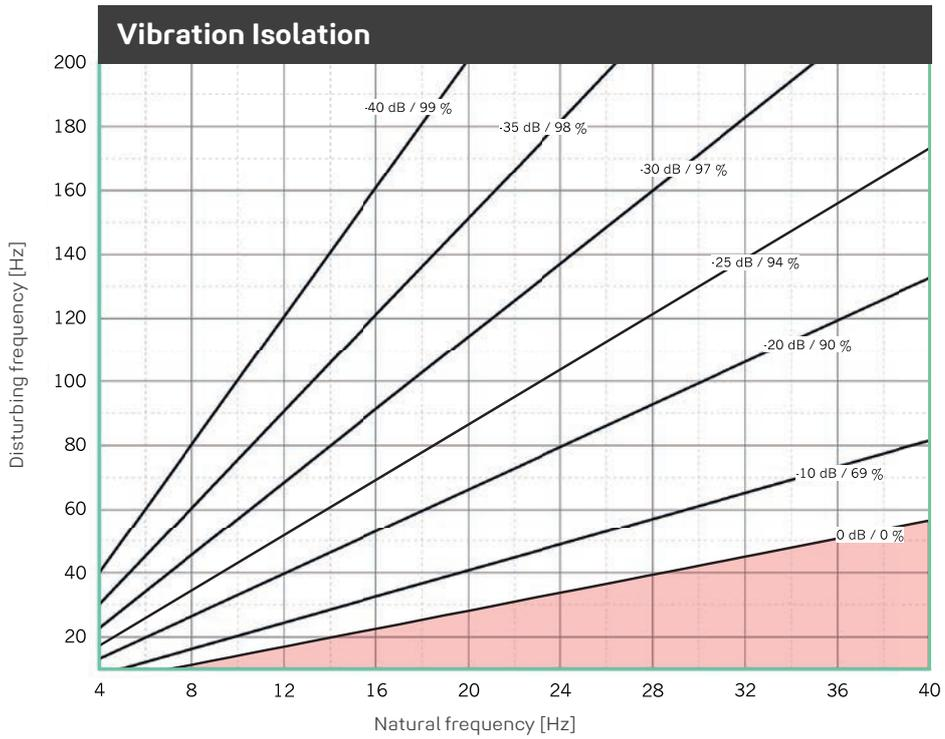
Illustration of the isolation efficiency of a single-degree-of-freedom system (SDOF system) on a rigid base with **REGUFOAM vibration 150plus**. Parameter: power transmission (insertion loss) in dB, isolation factor in %.
