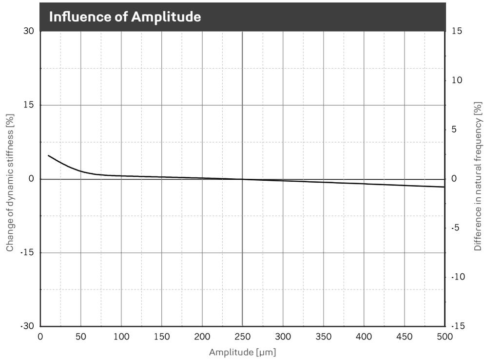
Change of the dynamic stiffness due to changes in amplitudes. Average for 5 Hz, 10 Hz and 40 Hz excitation. Sinusoidal excitation at a constant mean load of 0.055 N/mm<sup>2</sup>, dimensions of the specimens 300 x 300 x 25 mm. Natural frequency of a single-degree-of-freedom system (SDOF system) on a rigid base.
