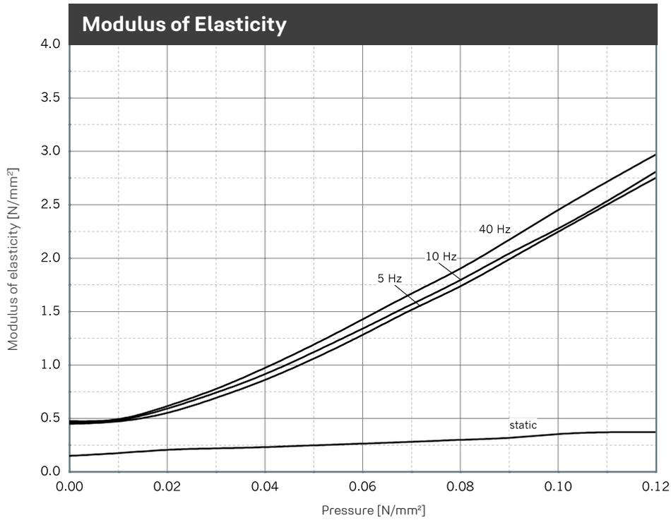
Illustration of the dynamic modulus of elasticity for sinusoidal excitation at a constant mean load and an amplitude of  $\pm 0.25$  mm. Dimensions of specimens 300 x 300 x 50 mm; static modulus of elasticity as a result of the tangent modulus of the spring characteristic. Tested in accordance with DIN 53513.
