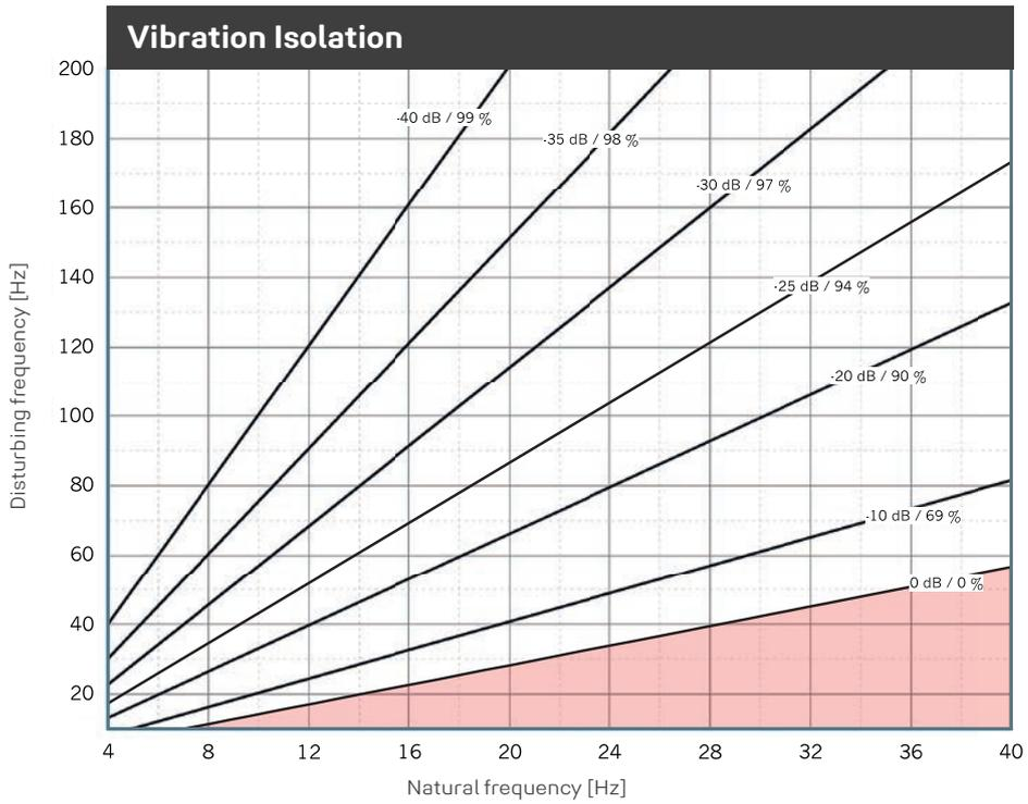
Illustration of the isolation efficiency of a single-degree-of-freedom system (SDOF system) on a rigid base with **REGUPOL vibration 400**. Parameter: power transmission (insertion loss) in dB, isolation factor in %.
