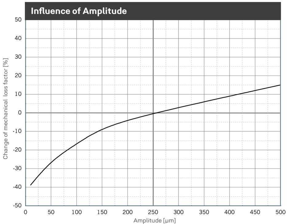
Change of the mechanical loss factor due to changes in amplitudes. Sinusoidal excitation at a constant mean load of 1.50 N/mm<sup>2</sup>, dimensions of the specimens 200 x 200 x 60 mm.
