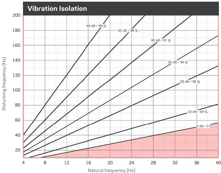
Illustration of the isolation efficiency of a single-degree-of-freedom system (SDOF system) on a rigid base with **REGUFOAM vibration 570plus**. Parameter: power transmission (insertion loss) in dB, isolation factor in %.
