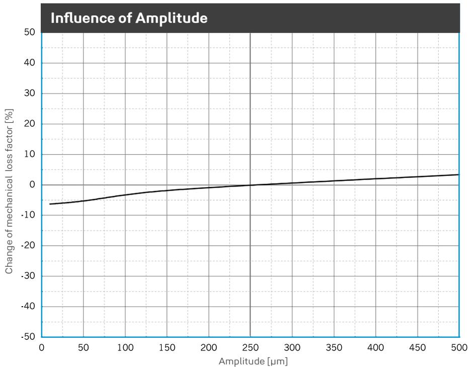
Change of the mechanical loss factor due to changes in amplitudes. Sinusoidal excitation at a constant mean load of 0.042 N/mm<sup>2</sup>, dimensions of the specimens 300 x 300 x 25 mm.
