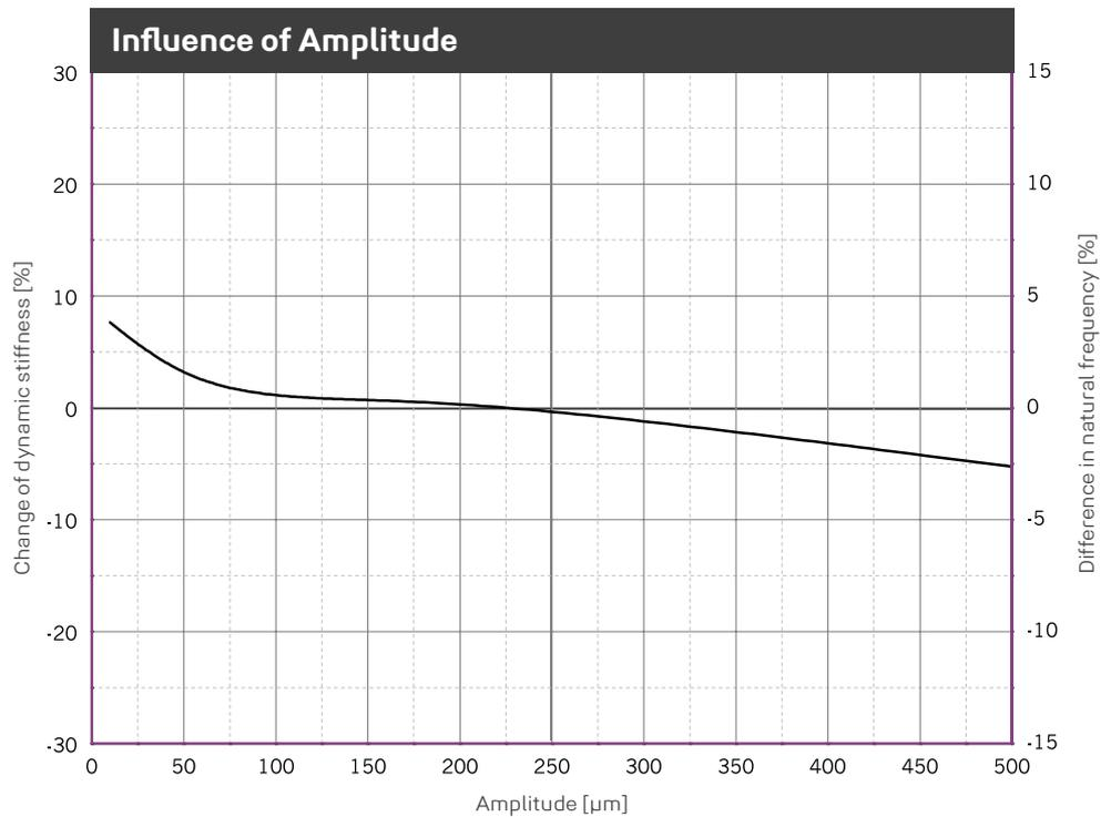
Change of the dynamic stiffness due to changes in amplitudes. Average for 5 Hz, 10 Hz and 40 Hz excitation. Sinusoidal excitation at a constant mean load of 0.028 N/mm<sup>2</sup>, dimensions of the specimens 300 x 300 x 25 mm. Natural frequency of a single-degree-of-freedom system (SDOF system) on a rigid base.
