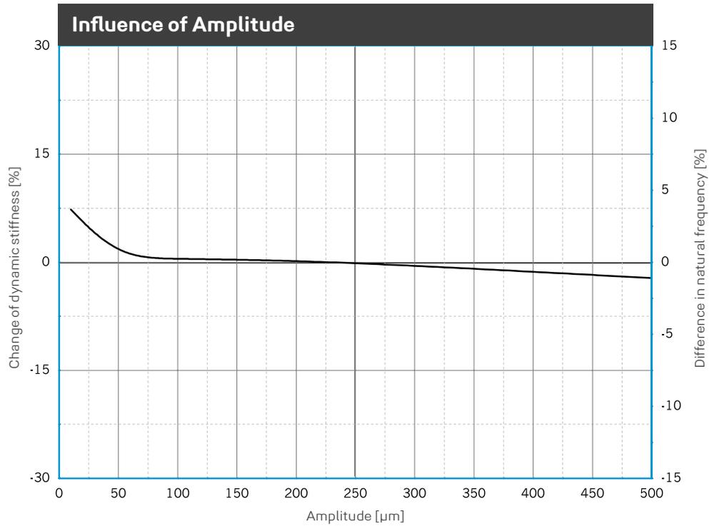
Change of the dynamic stiffness due to changes in amplitudes. Average for 5 Hz, 10 Hz and 40 Hz excitation. Sinusoidal excitation at a constant mean load of 0.042 N/mm<sup>2</sup>, dimensions of the specimens 300 x 300 x 25 mm. Natural frequency of a single-degree-of-freedom system (SDOF system) on a rigid base.
