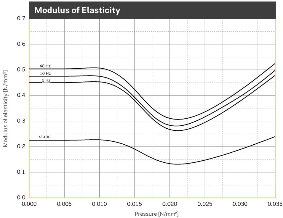
Illustration of the dynamic modulus of elasticity for sinusoidal excitation at a constant mean load and an amplitude of  $\pm 0.25$  mm. Dimensions of specimens  $300 \times 300 \times 25$  mm; static modulus of elasticity as a result of the tangent modulus of the spring characteristic. Tested in accordance with DIN 53513.
