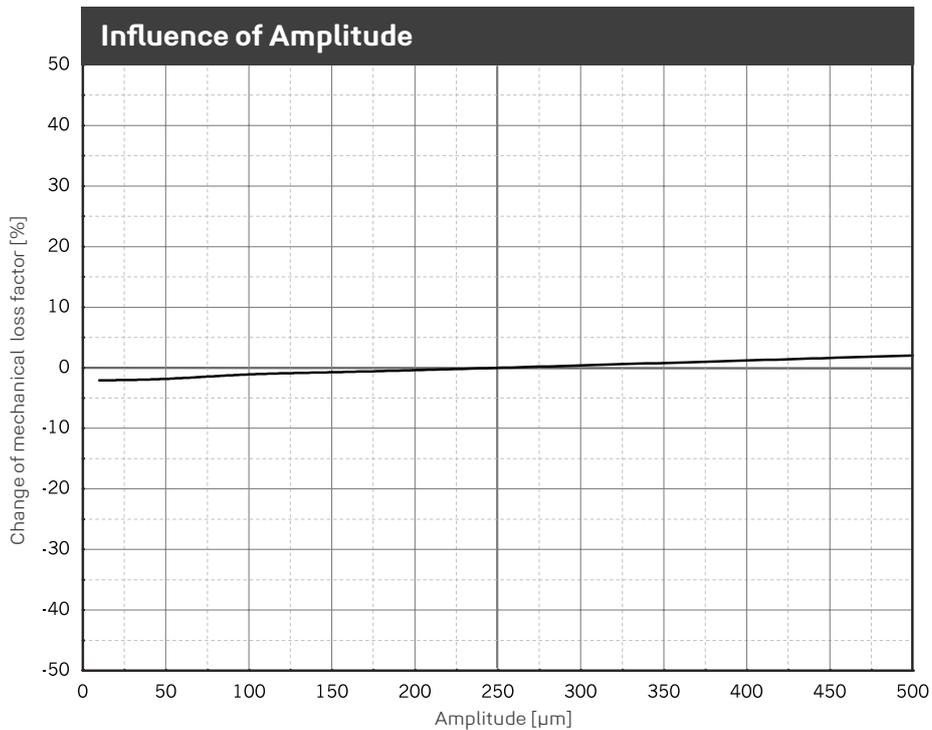
Change of the mechanical loss factor due to changes in amplitudes. Sinusoidal excitation at a constant mean load of 0.055 N/mm<sup>2</sup>, dimensions of the specimens 300 x 300 x 25 mm.
