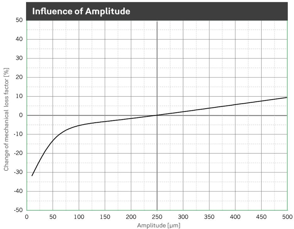
Change of the mechanical loss factor due to changes in amplitudes. Sinusoidal excitation at a constant mean load of 0.011 N/mm<sup>2</sup>, dimensions of the specimens 300 x 300 x 25 mm.
