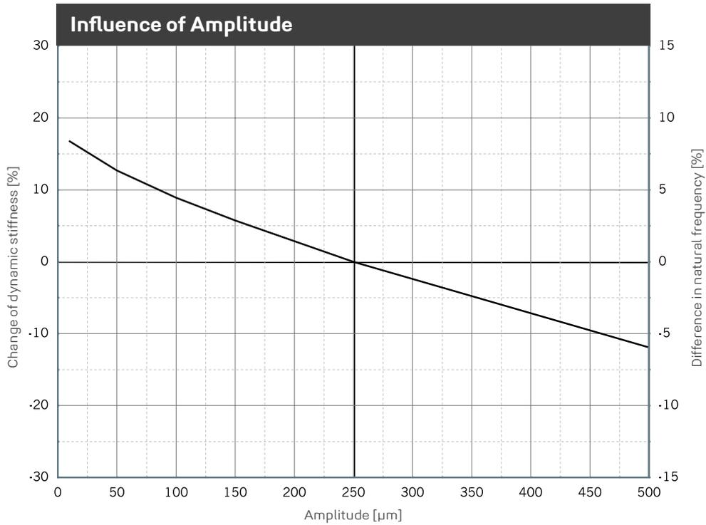
Change of the dynamic stiffness due to changes in amplitudes. Average for 5 Hz, 10 Hz and 40 Hz excitation. Sinusoidal excitation at a constant mean load of 0.10 N/mm<sup>2</sup>, dimensions of the specimens 300 x 300 x 60 mm. Natural frequency of a single-degree-of-freedom system (SDOF system) on a rigid base.
