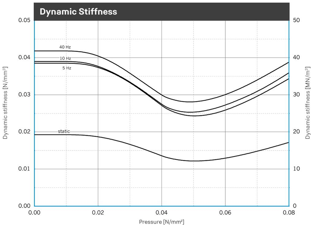
Illustration of the dynamic stiffness for sinusoidal excitation at a constant mean load and an amplitude of  $\pm 0.25$  mm. Dimensions of specimens  $300 \times 300 \times 25$  mm; static stiffness as a result of the tangent modulus of the spring characteristic. Tested in accordance with DIN 53513.
