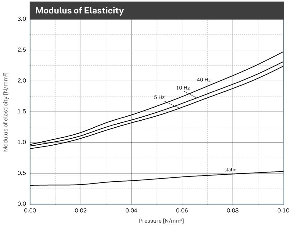
Illustration of the dynamic modulus of elasticity for sinusoidal excitation at a constant mean load and an amplitude of  $\pm 0.25$  mm. Dimensions of specimens 300 x 300 x 45 mm; static modulus of elasticity as a result of the tangent modulus of the spring characteristic. Tested in accordance with DIN 53513.
