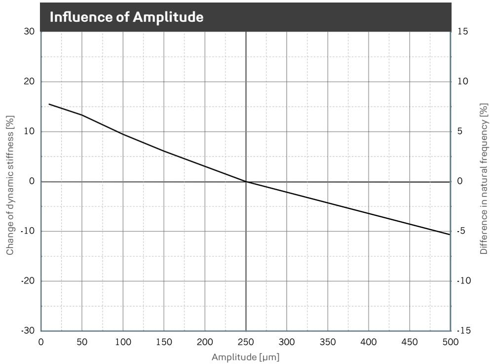
Change of the dynamic stiffness due to changes in amplitudes. Average for 5 Hz, 10 Hz and 40 Hz excitation. Sinusoidal excitation at a constant mean load of 1.50 N/mm<sup>2</sup>, dimensions of the specimens 200 x 200 x 60 mm. Natural frequency of a single-degree-of-freedom system (SDOF system) on a rigid base.
