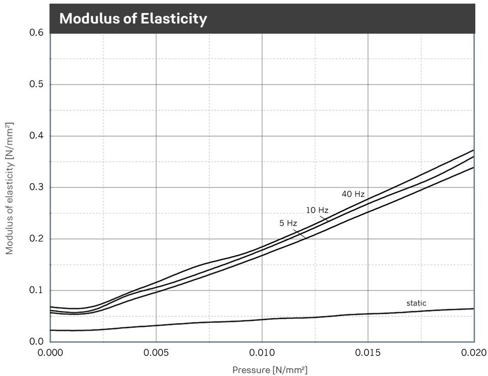
Illustration of the dynamic modulus of elasticity for sinusoidal excitation at a constant mean load and an amplitude of  $\pm 0.25$  mm. Dimensions of specimens 300 x 300 x 34 mm; static modulus of elasticity as a result of the tangent modulus of the spring characteristic. Tested in accordance with DIN 53513.
