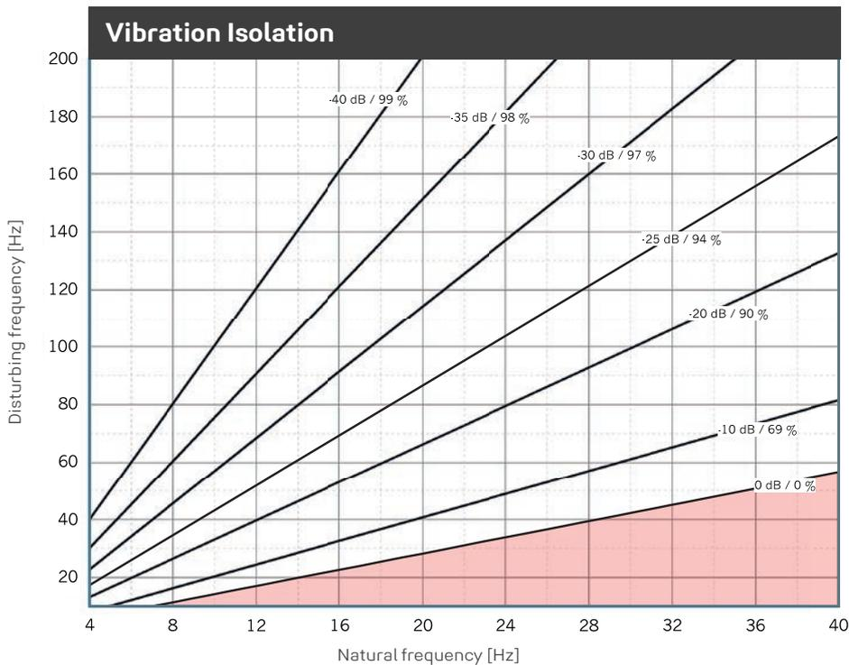
Illustration of the isolation efficiency of a single-degree-of-freedom system (SDOF system) on a rigid base with **REGUPOL vibration 550**. Parameter: power transmission (insertion loss) in dB, isolation factor in %.
