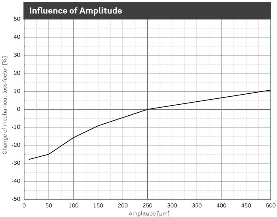
Change of the mechanical loss factor due to changes in amplitudes. Sinusoidal excitation at a constant mean load of 0.25 N/mm<sup>2</sup>, dimensions of the specimens 300 x 300 x 60 mm.
