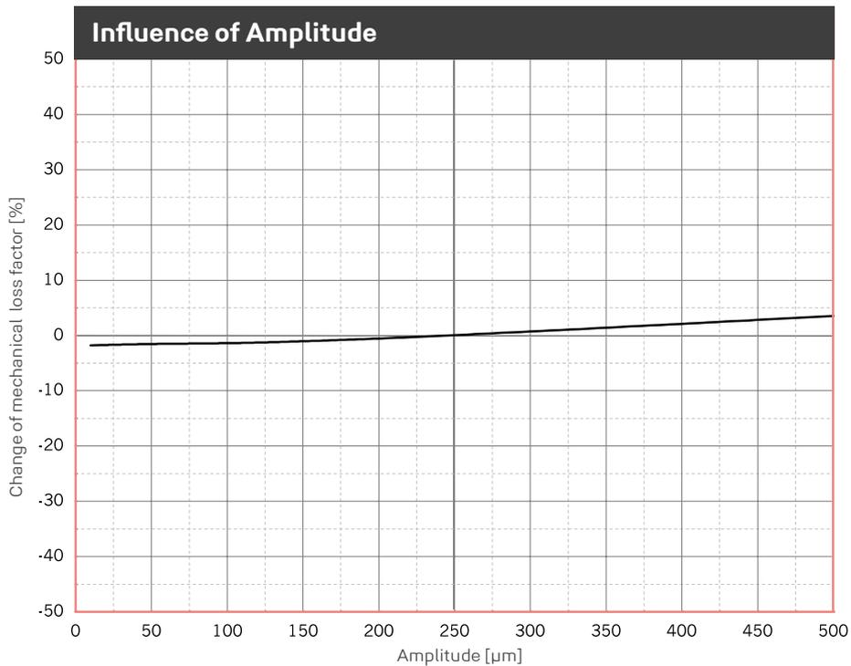
Change of the mechanical loss factor due to changes in amplitudes. Sinusoidal excitation at a constant mean load of 0.300 N/mm<sup>2</sup>, dimensions of the specimens 300 x 300 x 25 mm.
