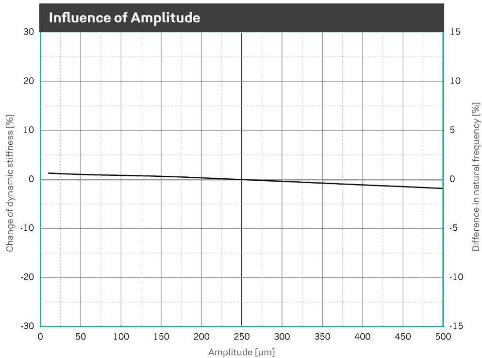
Change of the dynamic stiffness due to changes in amplitudes. Average for 5 Hz, 10 Hz and 40 Hz excitation. Sinusoidal excitation at a constant mean load of 0.450 N/mm<sup>2</sup>, dimensions of the specimens 300 x 300 x 25 mm. Natural frequency of a single-degree-of-freedom system (SDOF system) on a rigid base.
