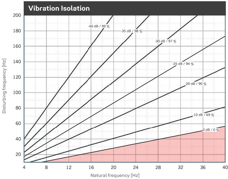
Illustration of the isolation efficiency of a single-degree-of-freedom system (SDOF system) on a rigid base with **REGUPOL vibration 200**. Parameter: power transmission (insertion loss) in dB, isolation factor in %.
