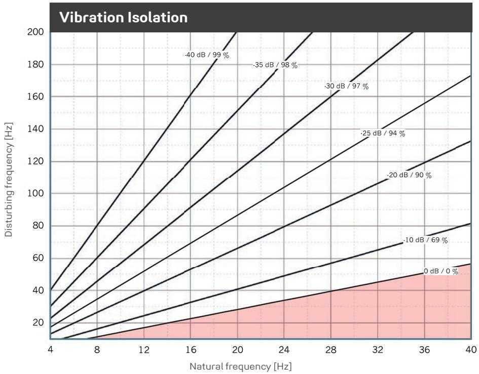
Illustration of the isolation efficiency of a single-degree-of-freedom system (SDOF system) on a rigid base with **REGUPOL vibration 800**. Parameter: power transmission (insertion loss) in dB, isolation factor in %.
