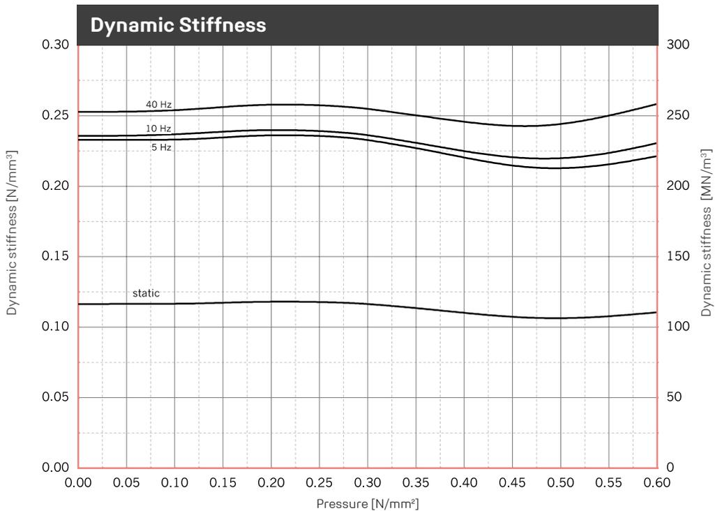
Illustration of the dynamic stiffness for sinusoidal excitation at a constant mean load and an amplitude of  $\pm 0.25$  mm. Dimensions of specimens  $300 \times 300 \times 25$  mm; static stiffness as a result of the tangent modulus of the spring characteristic. Tested in accordance with DIN 53513.
