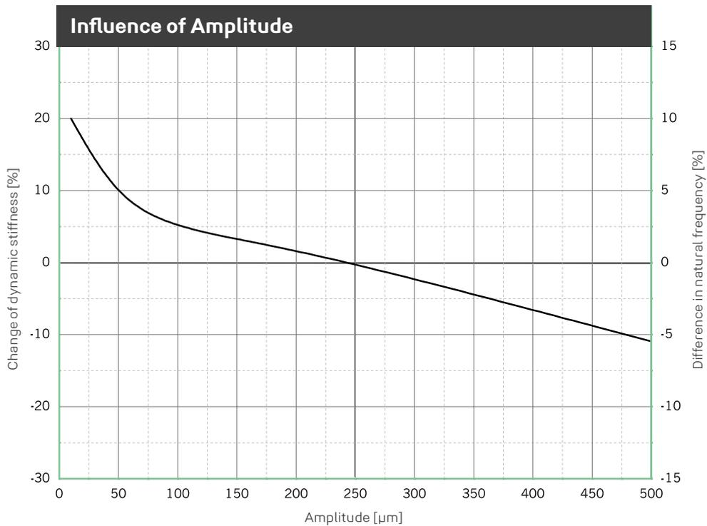
Change of the dynamic stiffness due to changes in amplitudes. Average for 5 Hz, 10 Hz and 40 Hz excitation. Sinusoidal excitation at a constant mean load of 0.011 N/mm<sup>2</sup>, dimensions of the specimens 300 x 300 x 25 mm. Natural frequency of a single-degree-of-freedom system (SDOF system) on a rigid base.
