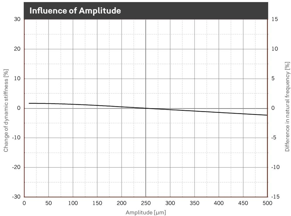
Change of the dynamic stiffness due to changes in amplitudes. Average for 5 Hz, 10 Hz and 40 Hz excitation. Sinusoidal excitation at a constant mean load of 0.850 N/mm<sup>2</sup>, dimensions of the specimens 250 x 250 x 50 mm. Natural frequency of a single-degree-of-freedom system (SDOF system) on a rigid base.
