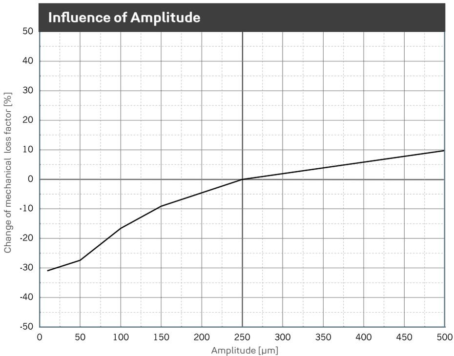
Change of the mechanical loss factor due to changes in amplitudes. Sinusoidal excitation at a constant mean load of 0.80 N/mm<sup>2</sup>, dimensions of the specimens 250 x 250 x 60 mm.
