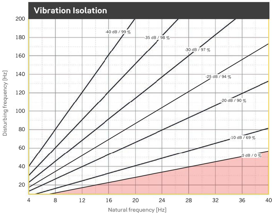
Illustration of the isolation efficiency of a single-degree-of-freedom system (SDOF system) on a rigid base with **REGUFOAM vibration 190plus**. Parameter: power transmission (insertion loss) in dB, isolation factor in %.
