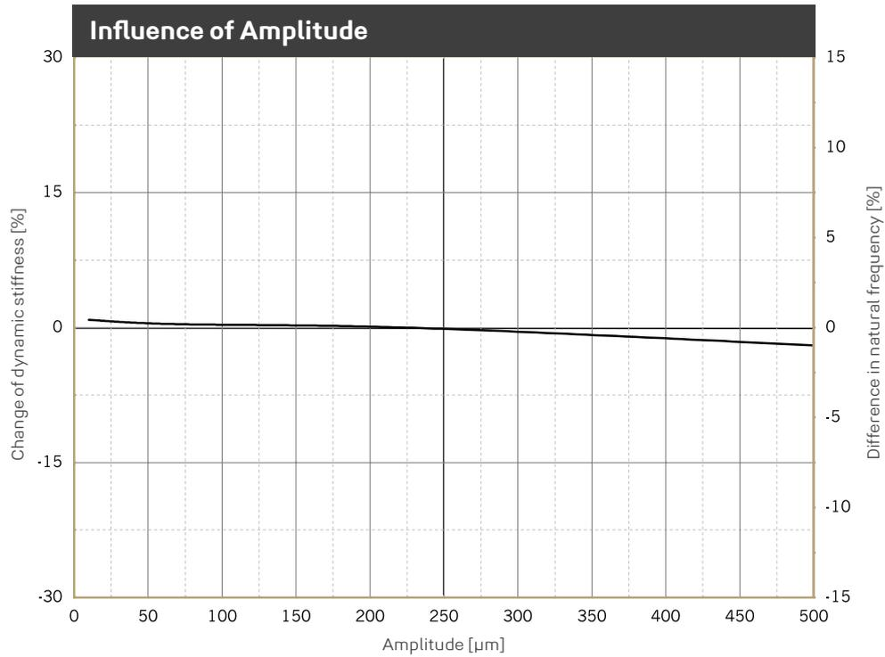
Change of the dynamic stiffness due to changes in amplitudes. Average for 5 Hz, 10 Hz and 40 Hz excitation. Sinusoidal excitation at a constant mean load of 0.220 N/mm<sup>2</sup>, dimensions of the specimens 300 x 300 x 25 mm. Natural frequency of a single-degree-of-freedom system (SDOF system) on a rigid base.
