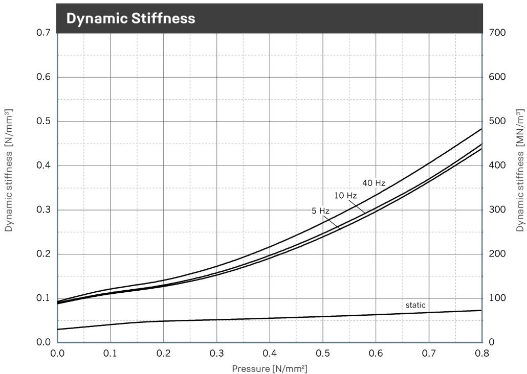
Illustration of the dynamic stiffness for sinusoidal excitation at a constant mean load and an amplitude of  $\pm 0.25$  mm. Dimensions of specimens  $250 \times 250 \times 40$  mm; static stiffness as a result of the tangent modulus of the spring characteristic. Tested in accordance with DIN 53513.
