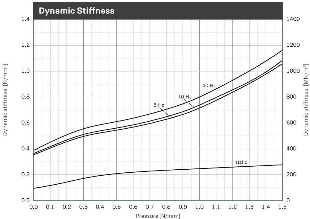
Illustration of the dynamic stiffness for sinusoidal excitation at a constant mean load and an amplitude of  $\pm 0.25$  mm. Dimensions of specimens  $200 \times 200 \times 40$  mm; static stiffness as a result of the tangent modulus of the spring characteristic. Tested in accordance with DIN 53513.
