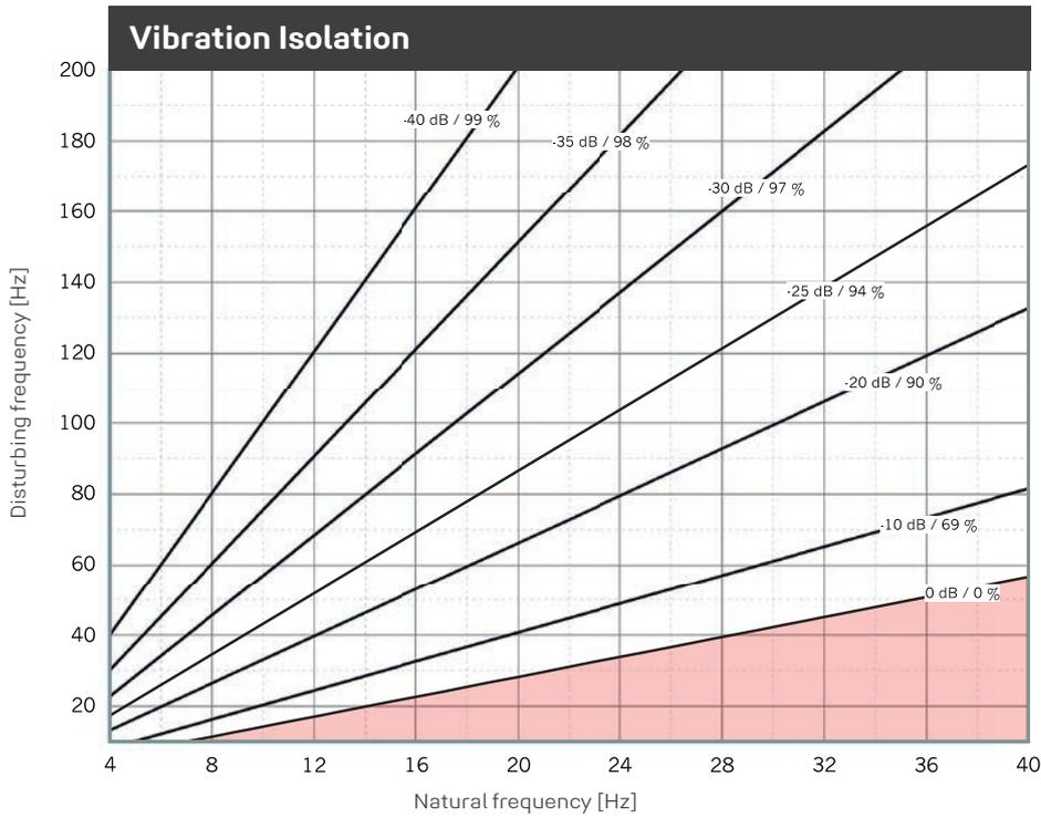
Illustration of the isolation efficiency of a single-degree-of-freedom system (SDOF system) on a rigid base with **REGUFOAM vibration 400plus**. Parameter: power transmission (insertion loss) in dB, isolation factor in %.
