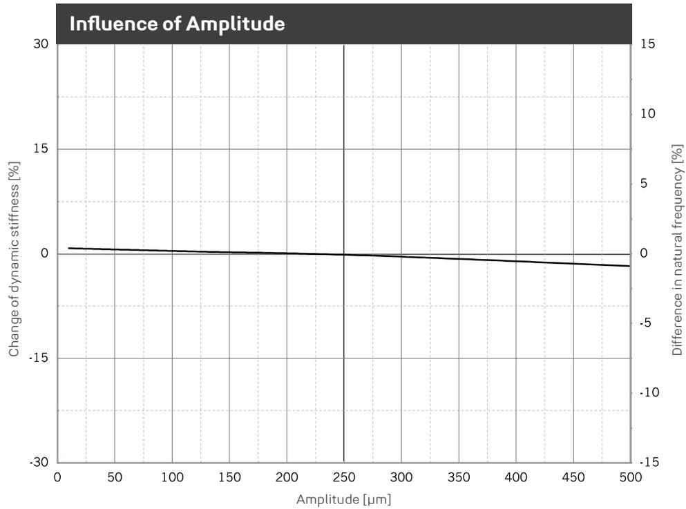
Change of the dynamic stiffness due to changes in amplitudes. Average for 5 Hz, 10 Hz and 40 Hz excitation. Sinusoidal excitation at a constant mean load of 0.110 N/mm<sup>2</sup>, dimensions of the specimens 300 x 300 x 25 mm. Natural frequency of a single-degree-of-freedom system (SDOF system) on a rigid base.
