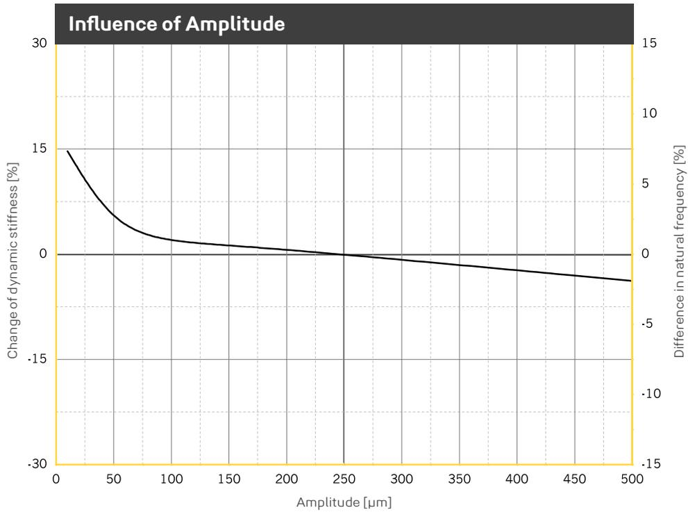
Change of the dynamic stiffness due to changes in amplitudes. Average for 5 Hz, 10 Hz and 40 Hz excitation. Sinusoidal excitation at a constant mean load of 0.018 N/mm<sup>2</sup>, dimensions of the specimens 300 x 300 x 25 mm. Natural frequency of a single-degree-of-freedom system (SDOF system) on a rigid base.
