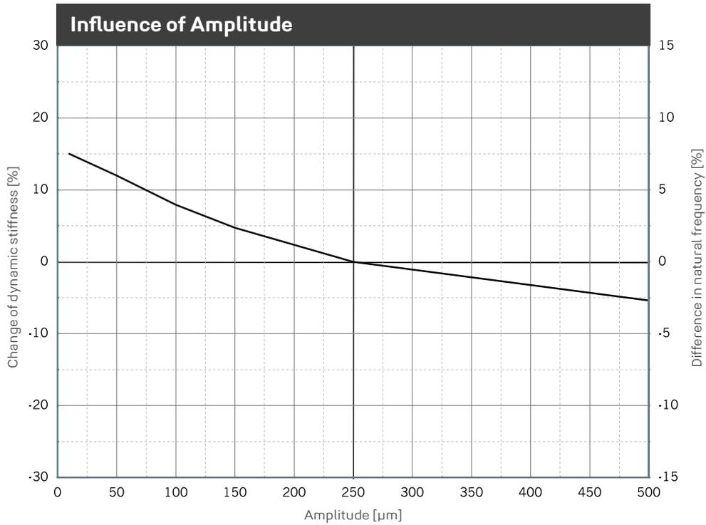
Change of the dynamic stiffness due to changes in amplitudes. Average for 5 Hz, 10 Hz and 40 Hz excitation. Sinusoidal excitation at a constant mean load of 0.011 N/mm<sup>2</sup>, dimensions of the specimens 300 x 300 x 51 mm. Natural frequency of a single-degree-of-freedom system (SDOF system) on a rigid base.
