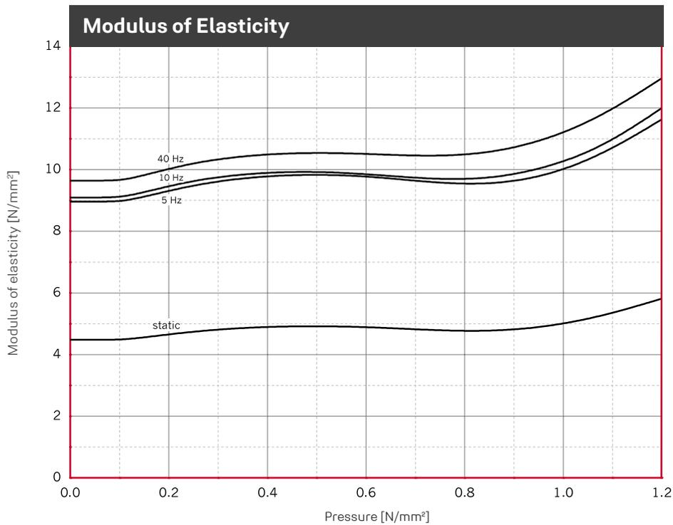
Illustration of the dynamic modulus of elasticity for sinusoidal excitation at a constant mean load and an amplitude of  $\pm 0.25$  mm. Dimensions of specimens 250 x 250 x 25 mm; static modulus of elasticity as a result of the tangent modulus of the spring characteristic. Tested in accordance with DIN 53513.
