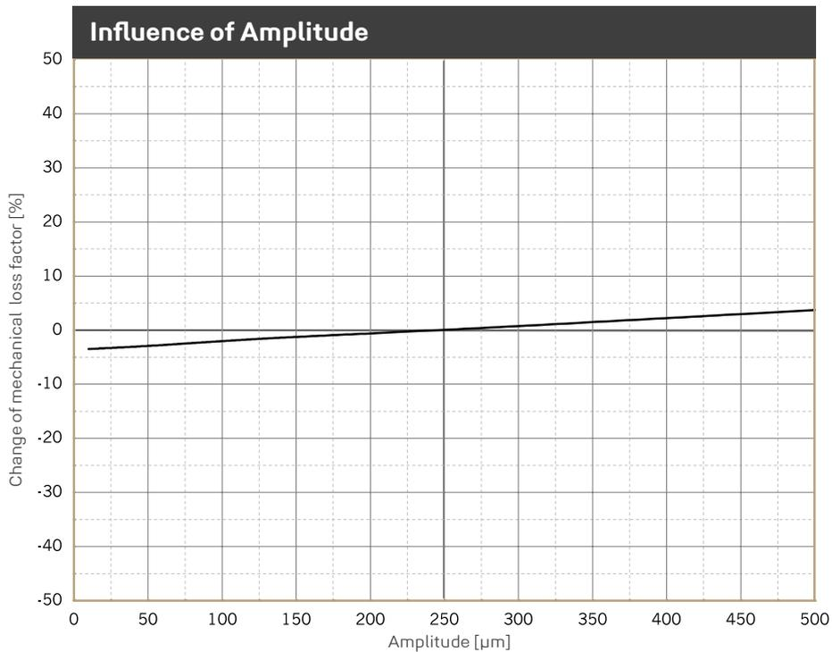
Change of the mechanical loss factor due to changes in amplitudes. Sinusoidal excitation at a constant mean load of 0.220 N/mm<sup>2</sup>, dimensions of the specimens 300 x 300 x 25 mm.
