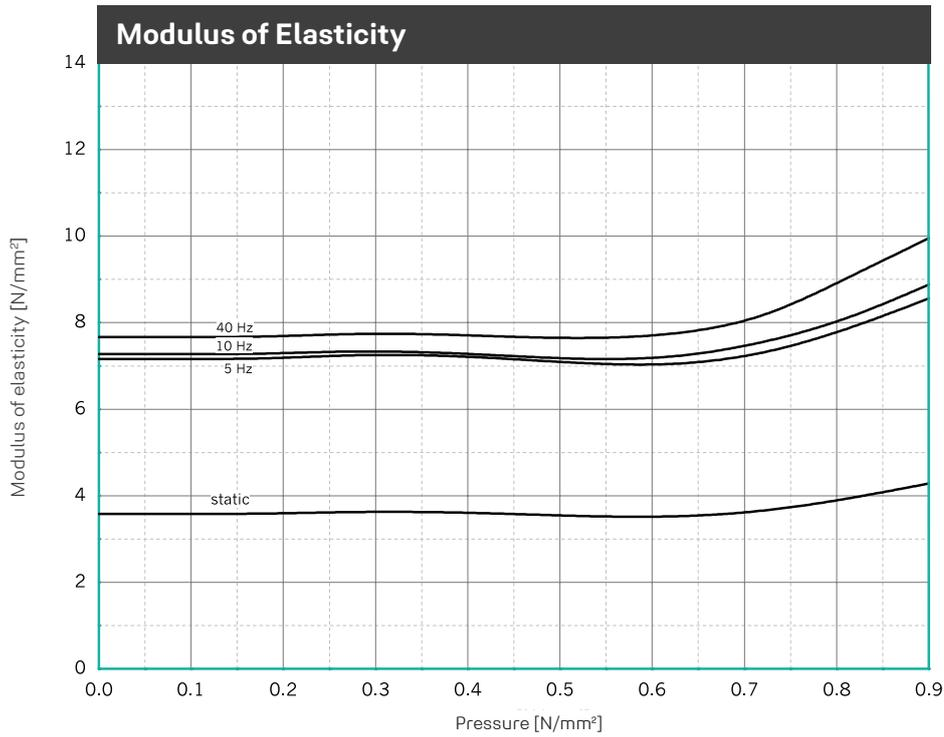
Illustration of the dynamic modulus of elasticity for sinusoidal excitation at a constant mean load and an amplitude of  $\pm 0.25$  mm. Dimensions of specimens 300 x 300 x 25 mm; static modulus of elasticity as a result of the tangent modulus of the spring characteristic. Tested in accordance with DIN 53513.
