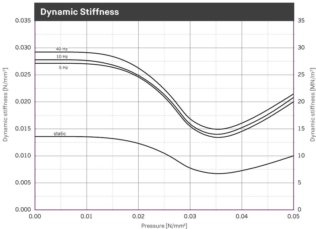
Illustration of the dynamic stiffness for sinusoidal excitation at a constant mean load and an amplitude of  $\pm 0.25$  mm. Dimensions of specimens 300 x 300 x 25 mm; static stiffness as a result of the tangent modulus of the spring characteristic. Tested in accordance with DIN 53513.
