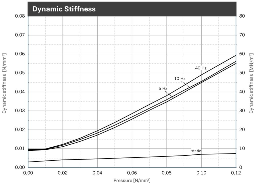
Illustration of the dynamic stiffness for sinusoidal excitation at a constant mean load and an amplitude of  $\pm 0.25$  mm. Dimensions of specimens 300 x 300 x 50 mm; static stiffness as a result of the tangent modulus of the spring characteristic. Tested in accordance with DIN 53513.
