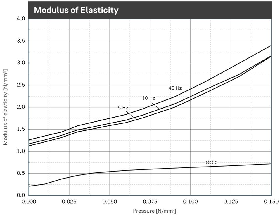
Illustration of the dynamic modulus of elasticity for sinusoidal excitation at a constant mean load and an amplitude of  $\pm 0.25$  mm. Dimensions of specimens  $300 \times 300 \times 45$  mm; static modulus of elasticity as a result of the tangent modulus of the spring characteristic. Tested in accordance with DIN 53513.
