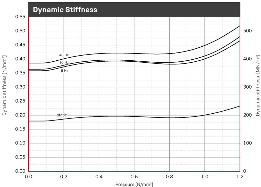
Illustration of the dynamic stiffness for sinusoidal excitation at a constant mean load and an amplitude of  $\pm 0.25$  mm. Dimensions of specimens  $250 \times 250 \times 25$  mm; static stiffness as a result of the tangent modulus of the spring characteristic. Tested in accordance with DIN 53513.
