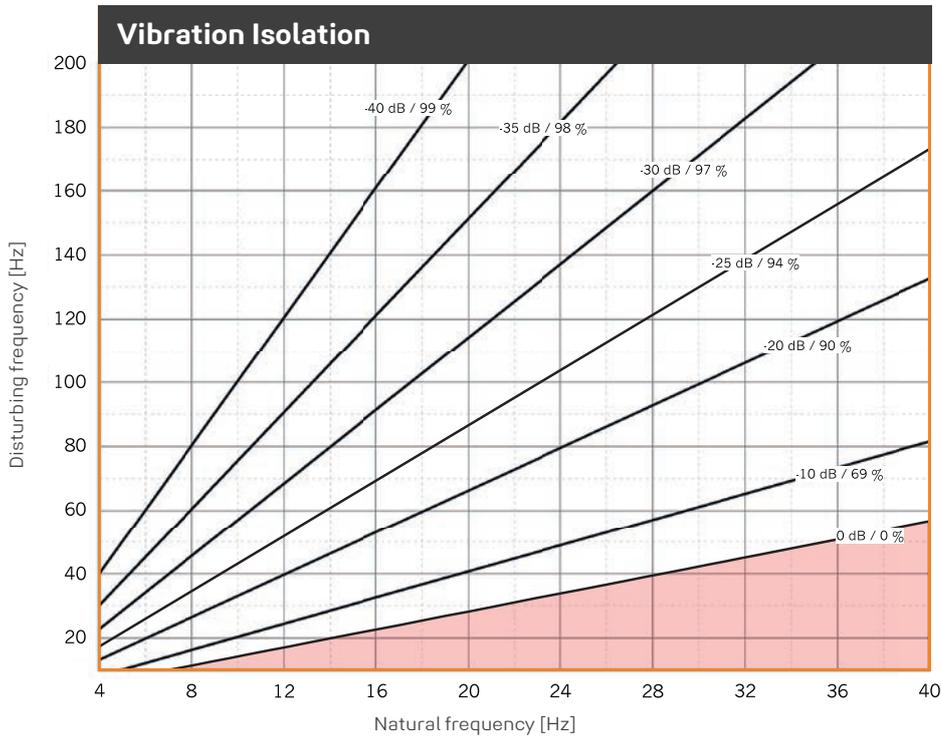
Illustration of the isolation efficiency of a single-degree-of-freedom system (SDOF system) on a rigid base with **REGUFOAM vibration 990plus**. Parameter: power transmission (insertion loss) in dB, isolation factor in %.
