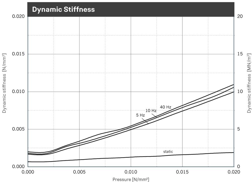
Illustration of the dynamic stiffness for sinusoidal excitation at a constant mean load and an amplitude of  $\pm 0.25$  mm. Dimensions of specimens 300 x 300 x 34 mm; static stiffness as a result of the tangent modulus of the spring characteristic. Tested in accordance with DIN 53513.
