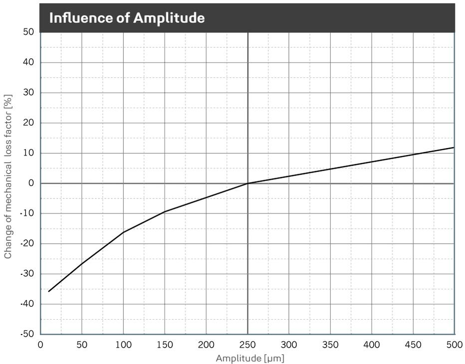
Change of the mechanical loss factor due to changes in amplitudes. Sinusoidal excitation at a constant mean load of 0.10 N/mm<sup>2</sup>, dimensions of the specimens 300 x 300 x 60 mm.
