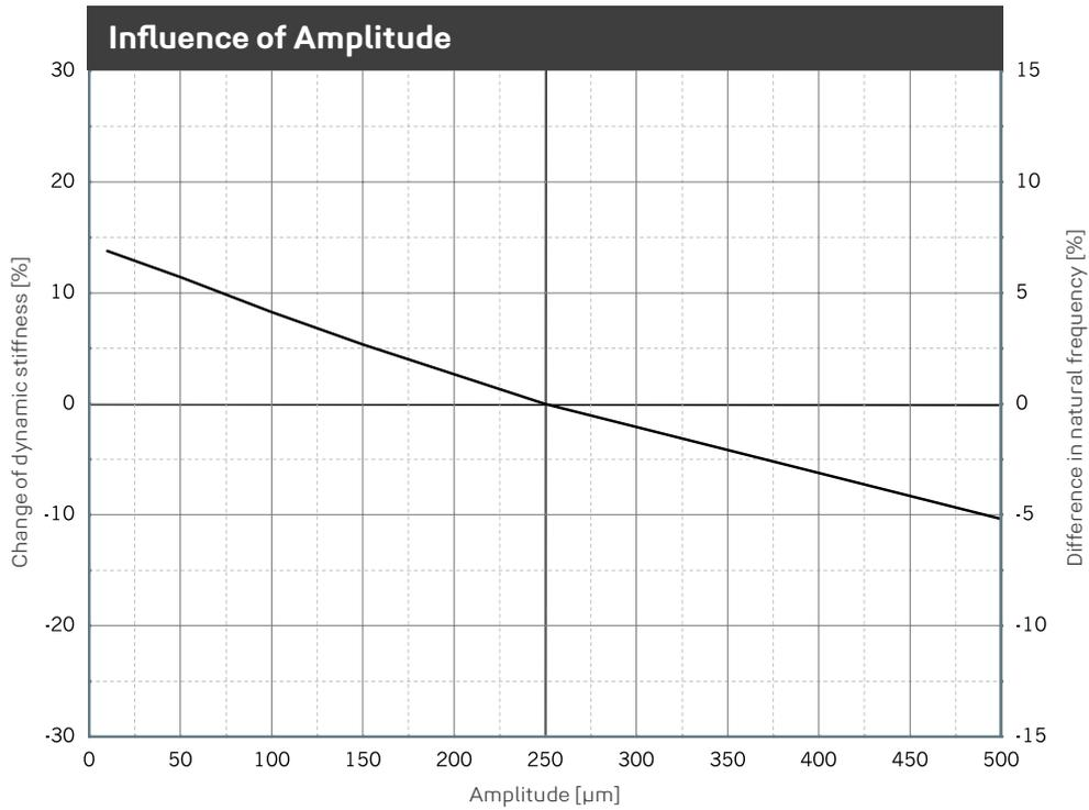
Change of the dynamic stiffness due to changes in amplitudes. Average for 5 Hz, 10 Hz and 40 Hz excitation. Sinusoidal excitation at a constant mean load of 0.25 N/mm<sup>2</sup>, dimensions of the specimens 300 x 300 x 60 mm. Natural frequency of a single-degree-of-freedom system (SDOF system) on a rigid base.
