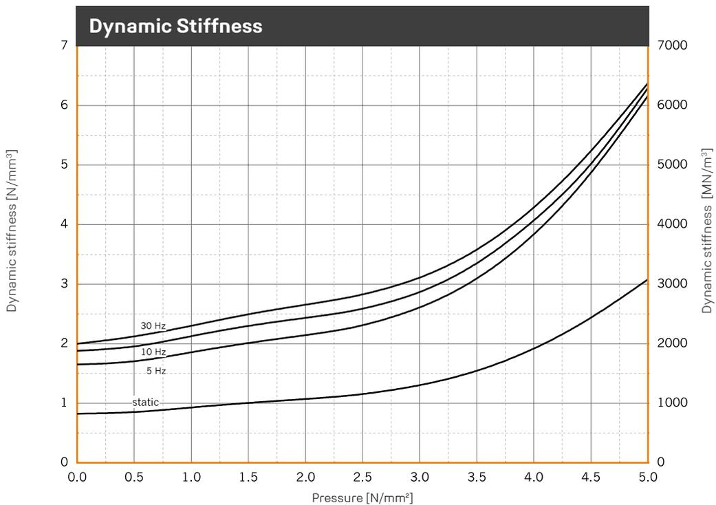
Illustration of the dynamic stiffness for sinusoidal excitation at a constant mean load and an amplitude of  $\pm 0.10$  mm. Dimensions of specimens  $125 \times 125 \times 25$  mm; static stiffness as a result of the tangent modulus of the spring characteristic. Tested in accordance with DIN 53513.
