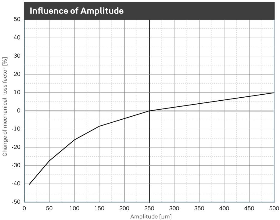
Change of the mechanical loss factor due to changes in amplitudes. Sinusoidal excitation at a constant mean load of 0.05 N/mm<sup>2</sup>, dimensions of the specimens 300 x 300 x 51 mm.
