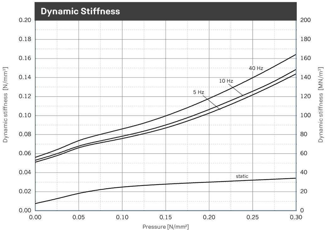
Illustration of the dynamic stiffness for sinusoidal excitation at a constant mean load and an amplitude of  $\pm 0.25$  mm. Dimensions of specimens  $300 \times 300 \times 45$  mm; static stiffness as a result of the tangent modulus of the spring characteristic. Tested in accordance with DIN 53513.
