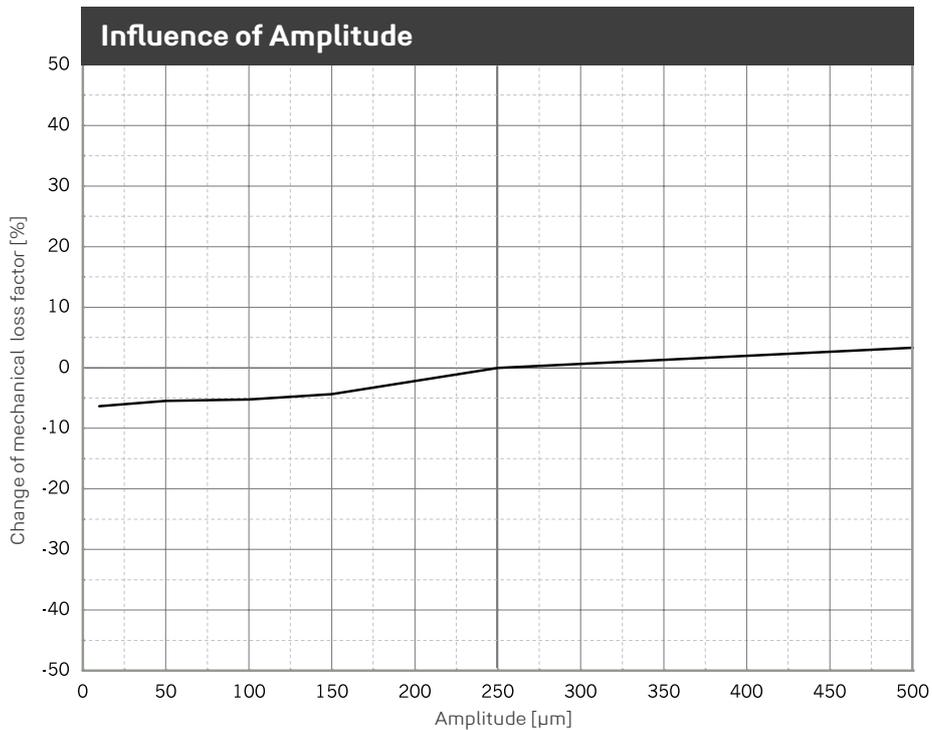
Change of the mechanical loss factor due to changes in amplitudes. Sinusoidal excitation at a constant mean load of 0.110 N/mm<sup>2</sup>, dimensions of the specimens 300 x 300 x 25 mm.
