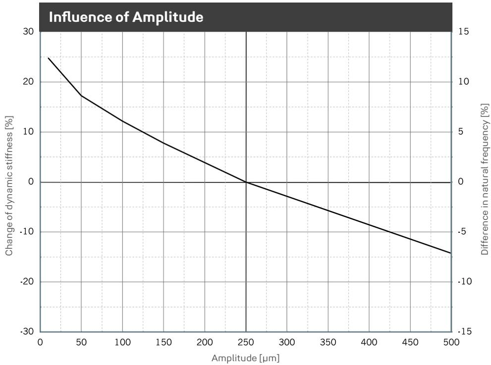
Change of the dynamic stiffness due to changes in amplitudes. Average for 5 Hz, 10 Hz and 40 Hz excitation. Sinusoidal excitation at a constant mean load of 0.05 N/mm<sup>2</sup>, dimensions of the specimens 300 x 300 x 51 mm. Natural frequency of a single-degree-of-freedom system (SDOF system) on a rigid base.
