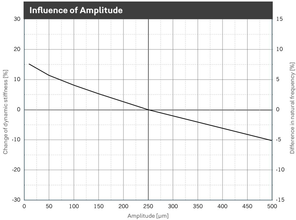
Change of the dynamic stiffness due to changes in amplitudes. Average for 5 Hz, 10 Hz and 40 Hz excitation. Sinusoidal excitation at a constant mean load of 0.10 N/mm<sup>2</sup>, dimensions of the specimens 300 x 300 x 50 mm. Natural frequency of a single-degree-of-freedom system (SDOF system) on a rigid base.
