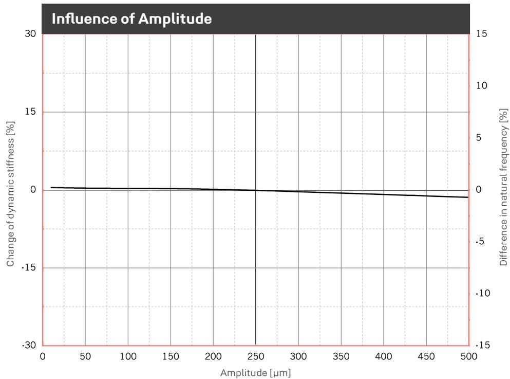
Change of the dynamic stiffness due to changes in amplitudes. Average for 5 Hz, 10 Hz and 40 Hz excitation. Sinusoidal excitation at a constant mean load of 0.300 N/mm<sup>2</sup>, dimensions of the specimens 300 x 300 x 25 mm. Natural frequency of a single-degree-of-freedom system (SDOF system) on a rigid base.
