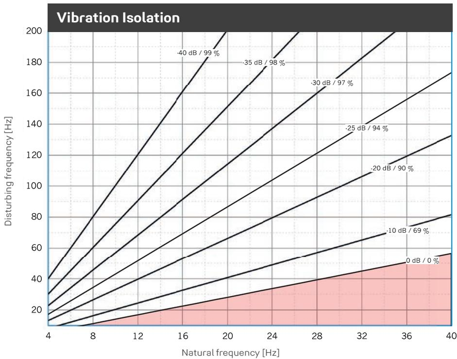
Illustration of the isolation efficiency of a single-degree-of-freedom system (SDOF system) on a rigid base with **REGUFOAM vibration 270plus**. Parameter: power transmission (insertion loss) in dB, isolation factor in %.
