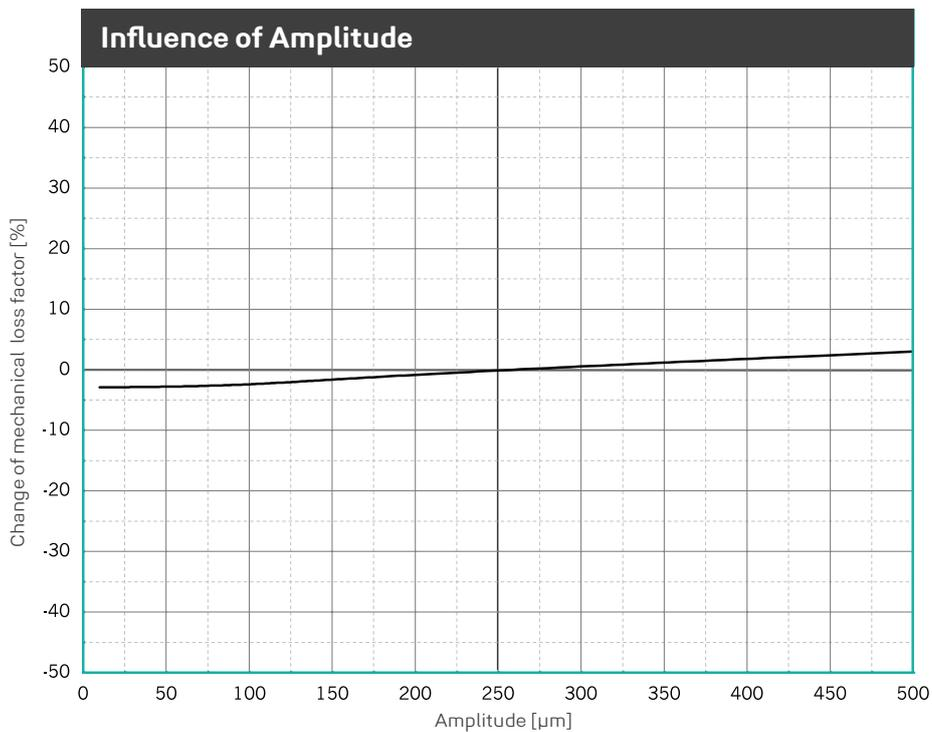
Change of the mechanical loss factor due to changes in amplitudes. Sinusoidal excitation at a constant mean load of 0.450 N/mm<sup>2</sup>, dimensions of the specimens 300 x 300 x 25 mm.
