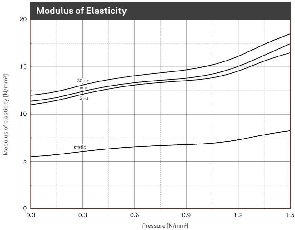
Illustration of the dynamic modulus of elasticity for sinusoidal excitation at a constant mean load and an amplitude of  $\pm 0.10$  mm. Dimensions of specimens 250 x 250 x 25 mm; static modulus of elasticity as a result of the tangent modulus of the spring characteristic. Tested in accordance with DIN 53513.
