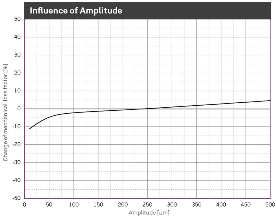
Change of the mechanical loss factor due to changes in amplitudes. Sinusoidal excitation at a constant mean load of 0.028 N/mm<sup>2</sup>, dimensions of the specimens 300 x 300 x 25 mm.
