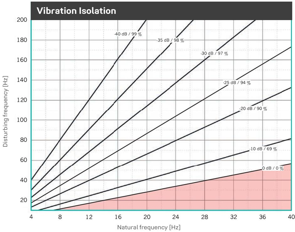
Illustration of the isolation efficiency of a single-degree-of-freedom system (SDOF system) on a rigid base with **REGUFOAM vibration 680plus**. Parameter: power transmission (insertion loss) in dB, isolation factor in %.
