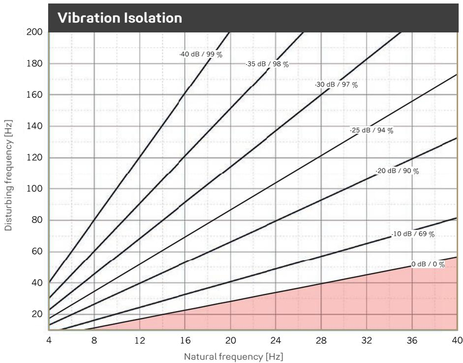
Illustration of the isolation efficiency of a single-degree-of-freedom system (SDOF system) on a rigid base with **REGUFOAM vibration 510plus**. Parameter: power transmission (insertion loss) in dB, isolation factor in %.
