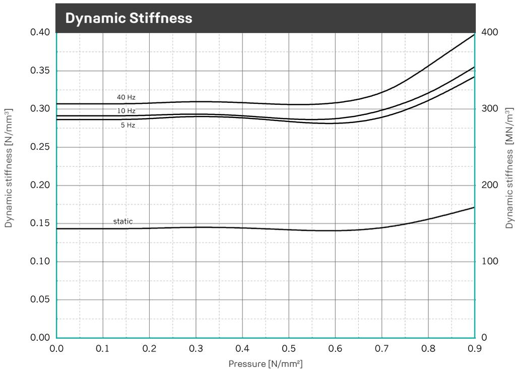
Illustration of the dynamic stiffness for sinusoidal excitation at a constant mean load and an amplitude of  $\pm 0.25$  mm. Dimensions of specimens 300 x 300 x 25 mm; static stiffness as a result of the tangent modulus of the spring characteristic. Tested in accordance with DIN 53513.
