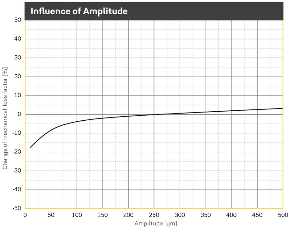
Change of the mechanical loss factor due to changes in amplitudes. Sinusoidal excitation at a constant mean load of 0.018 N/mm<sup>2</sup>, dimensions of the specimens 300 x 300 x 25 mm.
