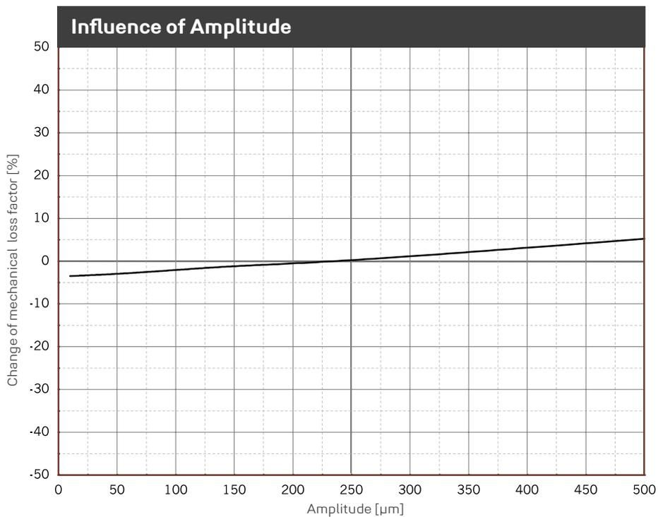
Change of the mechanical loss factor due to changes in amplitudes. Sinusoidal excitation at a constant mean load of 0.850 N/mm<sup>2</sup>, dimensions of the specimens 250 x 250 x 25 mm.
