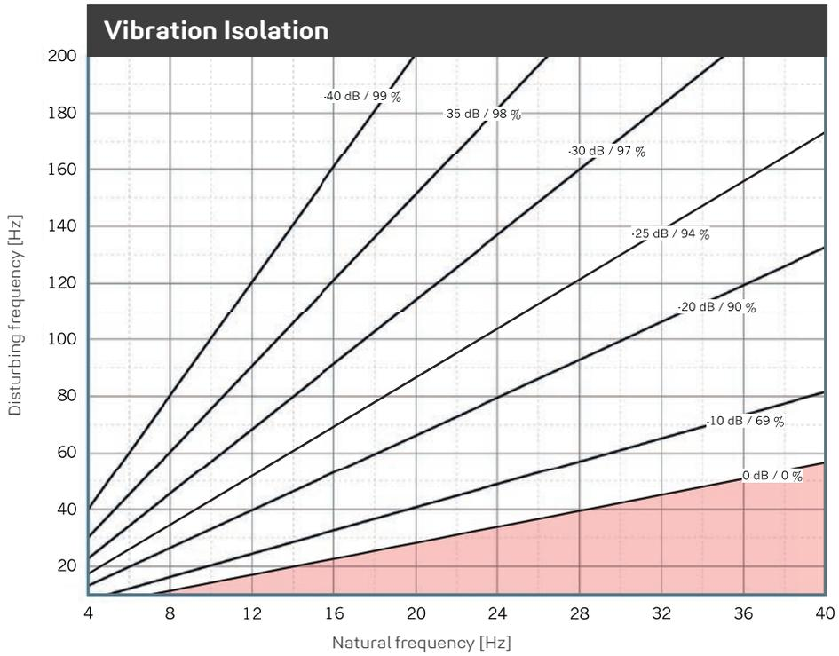
Illustration of the isolation efficiency of a single-degree-of-freedom system (SDOF system) on a rigid base with **REGUPOL vibration 300**. Parameter: power transmission (insertion loss) in dB, isolation factor in %.
