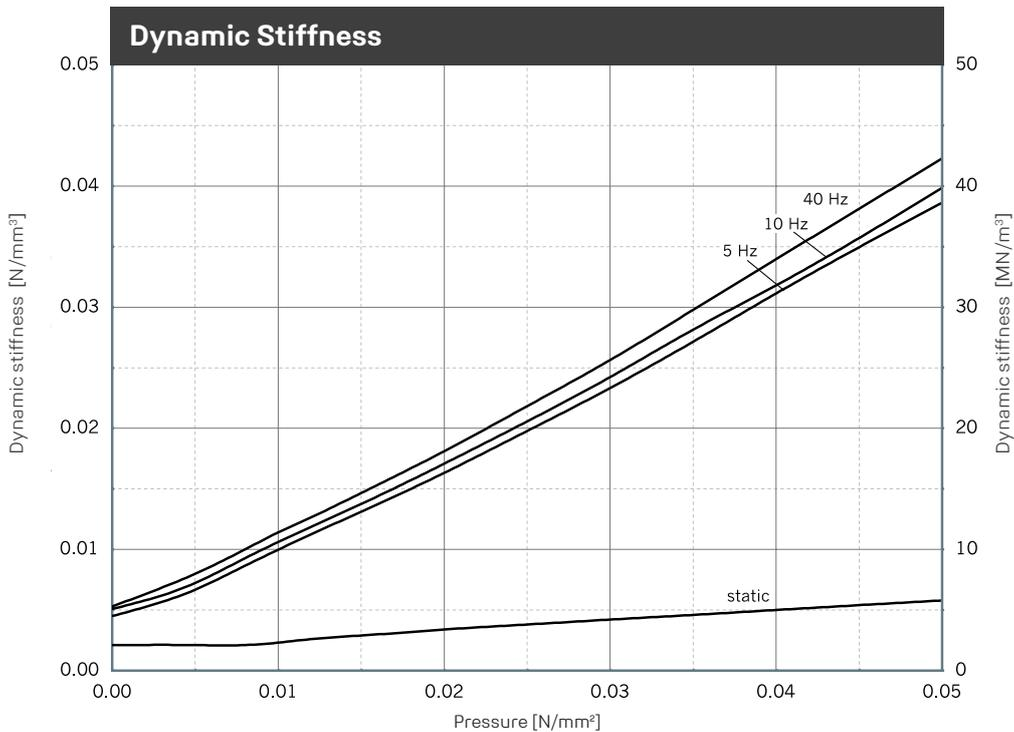
Illustration of the dynamic stiffness for sinusoidal excitation at a constant mean load and an amplitude of  $\pm 0.25$  mm. Dimensions of specimens 300 x 300 x 34 mm; static stiffness as a result of the tangent modulus of the spring characteristic. Tested in accordance with DIN 53513.
