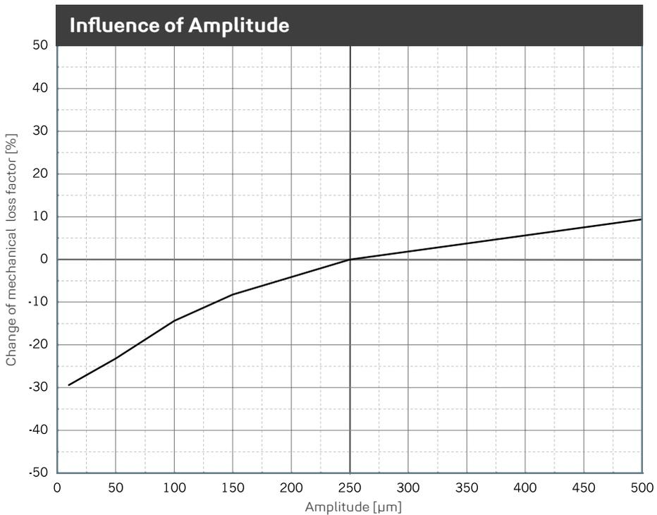
Change of the mechanical loss factor due to changes in amplitudes. Sinusoidal excitation at a constant mean load of 0.10 N/mm<sup>2</sup>, dimensions of the specimens 300 x 300 x 50 mm.
