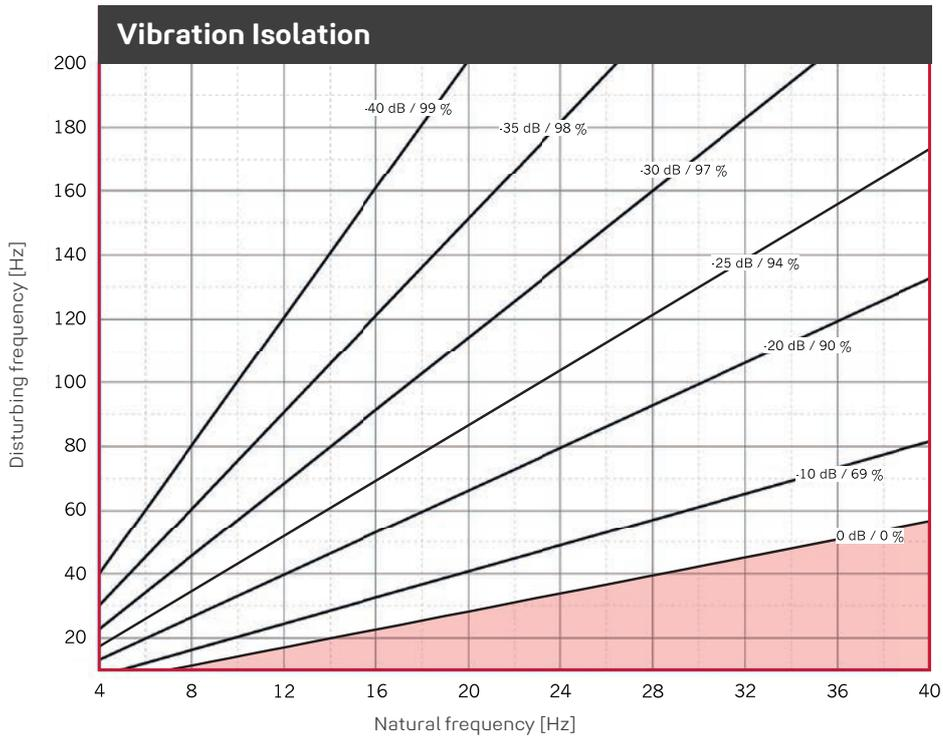
Illustration of the isolation efficiency of a single-degree-of-freedom system (SDOF system) on a rigid base with **REGUFOAM vibration 740plus**. Parameter: power transmission (insertion loss) in dB, isolation factor in %.
