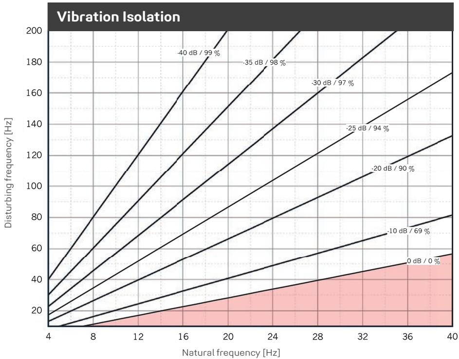
Illustration of the isolation efficiency of a single-degree-of-freedom system (SDOF system) on a rigid base with **REGUFOAM vibration 300plus**. Parameter: power transmission (insertion loss) in dB, isolation factor in %.
