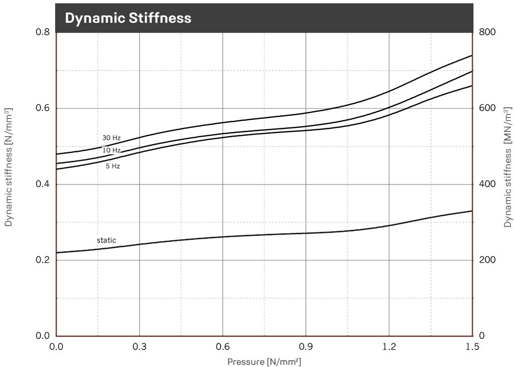
Illustration of the dynamic stiffness for sinusoidal excitation at a constant mean load and an amplitude of  $\pm 0.10$  mm. Dimensions of specimens 250 x 250 x 25 mm; static stiffness as a result of the tangent modulus of the spring characteristic. Tested in accordance with DIN 53513.
