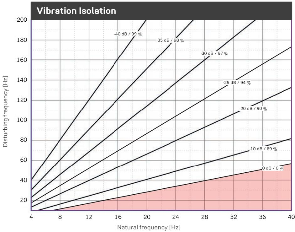
Illustration of the isolation efficiency of a single-degree-of-freedom system (SDOF system) on a rigid base with **REGUFOAM vibration 220plus**. Parameter: power transmission (insertion loss) in dB, isolation factor in %.
