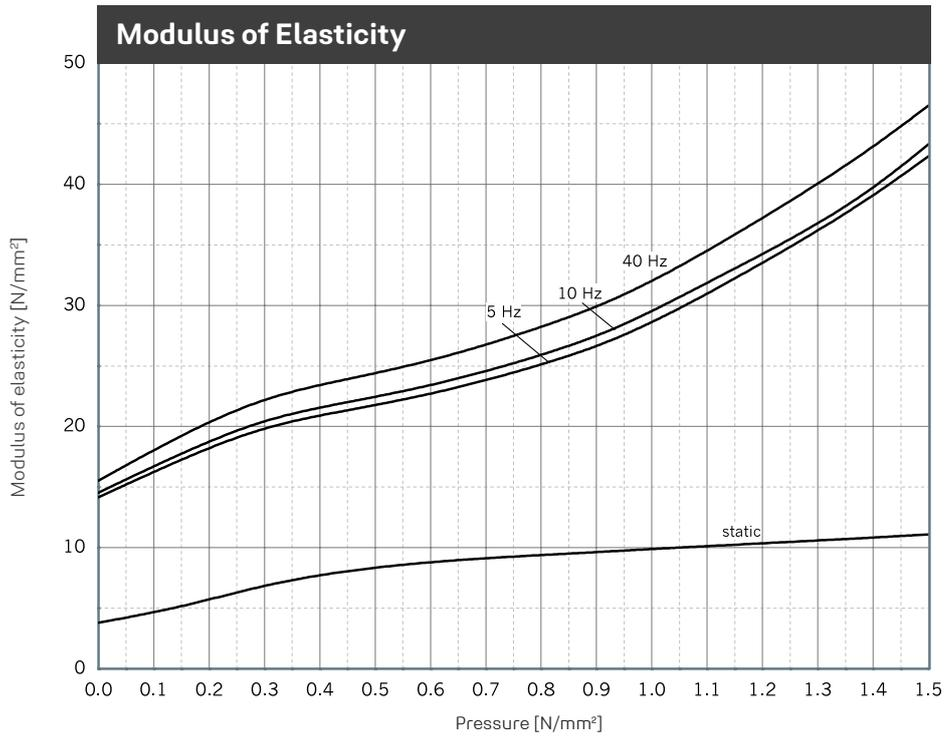
Illustration of the dynamic modulus of elasticity for sinusoidal excitation at a constant mean load and an amplitude of  $\pm 0.25$  mm. Dimensions of specimens  $200 \times 200 \times 40$  mm; static modulus of elasticity as a result of the tangent modulus of the spring characteristic. Tested in accordance with DIN 53513.
