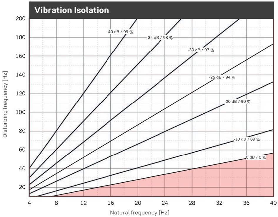
Illustration of the isolation efficiency of a single-degree-of-freedom system (SDOF system) on a rigid base with **REGUFOAM vibration 810plus**. Parameter: power transmission (insertion loss) in dB, isolation factor in %.
