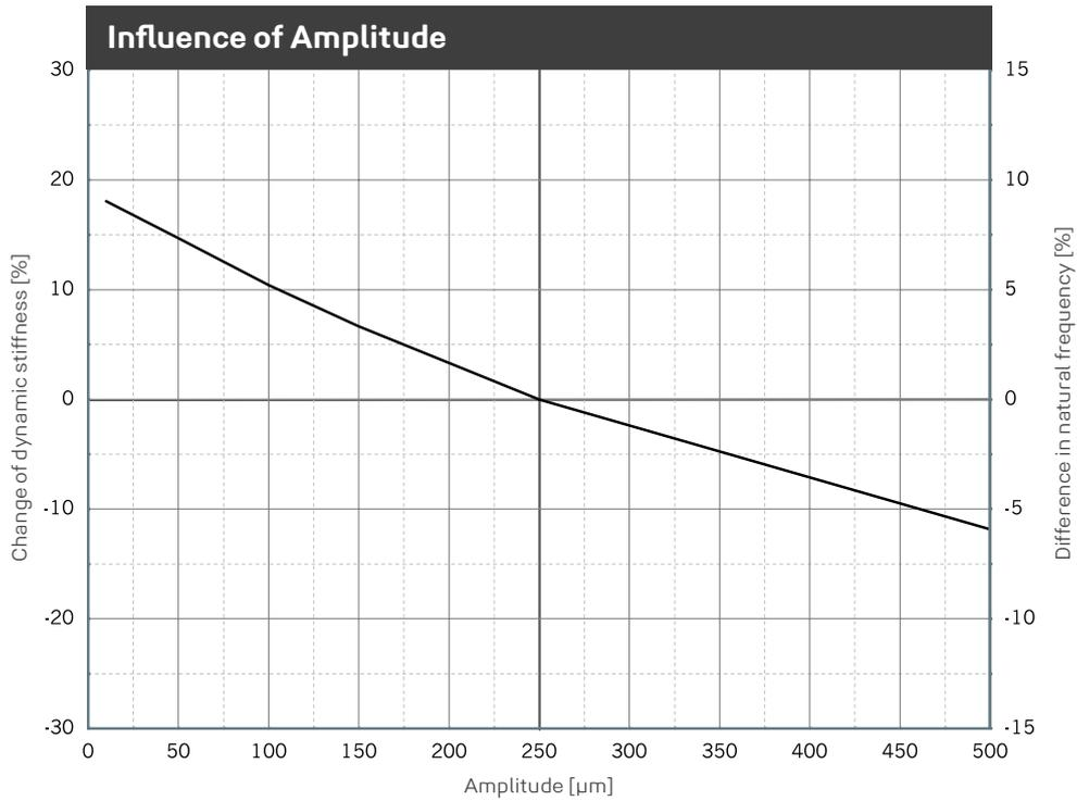
Change of the dynamic stiffness due to changes in amplitudes. Average for 5 Hz, 10 Hz and 40 Hz excitation. Sinusoidal excitation at a constant mean load of 0.80 N/mm<sup>2</sup>, dimensions of the specimens 250 x 250 x 60 mm. Natural frequency of a single-degree-of-freedom system (SDOF system) on a rigid base.
