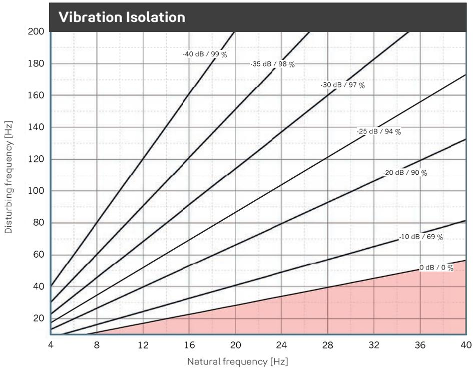
Illustration of the isolation efficiency of a single-degree-of-freedom system (SDOF system) on a rigid base with **REGUPOL vibration 1000**. Parameter: power transmission (insertion loss) in dB, isolation factor in %.
