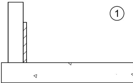
Tape or glue **REGUPOL perimeter isolation strips** in place, continuously on all adjoining structural elements, such as walls, columns, and protrusions.
