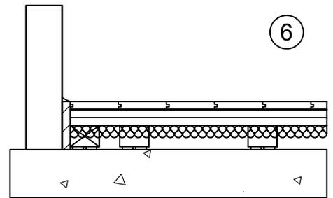
Trim excess **perimeter isolation strip** at or below the level of the finish flooring. Caulk using an acoustical sealant.
