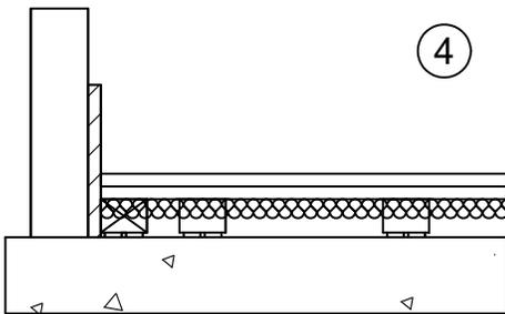
Install 2nd layer of 3/4" OSB or plywood over top of **soundpanel**, staggered, so that the seams do not line up. Glue and fasten with trowel, wood glue, 1-1/4" screws, 6" o.c. at perimeter, and 8" o.c. throughout.
