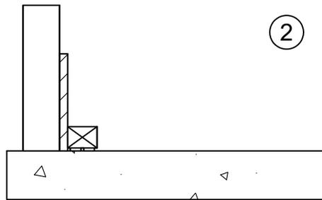
Place **REGUPOL soundpads** butt-joined to the perimeter of the room, around all structural elements. Individual **soundpads** should be spaced equal to or less than 16".
