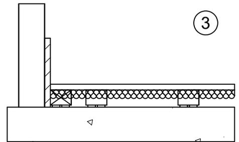
Place the first row of **soundpanel** starting in one corner of the room. Start the next row of **soundpanel** offset by 16". Cut the first **soundpanel** of every other row, then continue with full panels.
