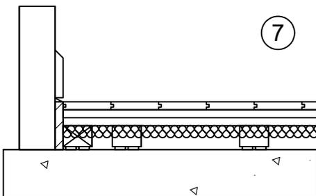
Leave a slight gap between the baseboard and the finished floor. Avoid any rigid connections between the isolated floating floor and adjacent structural elements.
