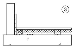
Tape or glue **REGUPOL perimeter isolation strips** in place, continuously on all adjoining strucutral elements, such as walls, columns, and protrusions.
